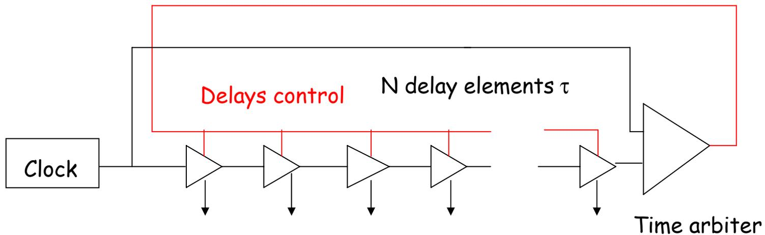
Clock feeds the digital delay line
