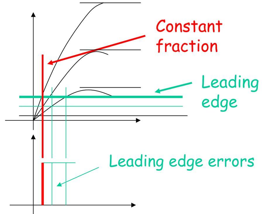
If pulse shape independent of amplitude, use Constant fraction
