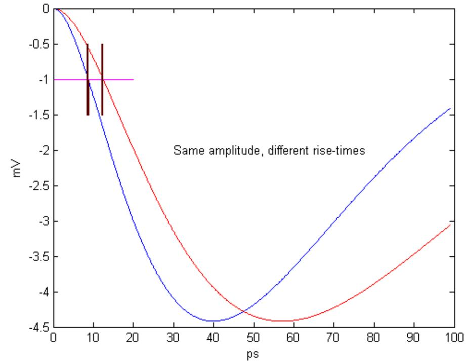
**Amplitude** and/or **Rise-time** spectra translate into **time spread**
