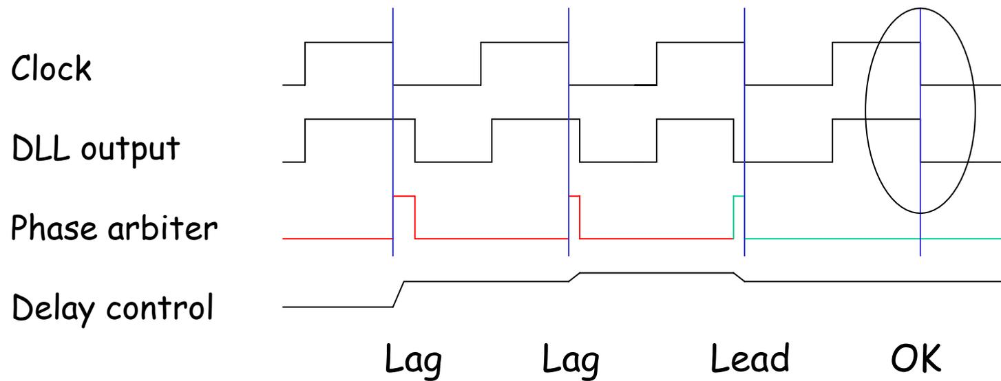
Feedback can be analog (RC filter) or digital using the TDC digital response itself
