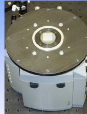
EMCCD camera with fiber taper and columnar-grown CsI(Tl) scintillator
