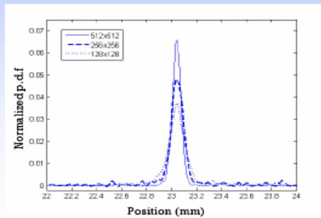
Measured line-spread functions with different binning
