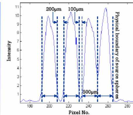
1-d profile of cutting through the four spheres on the right hand side
