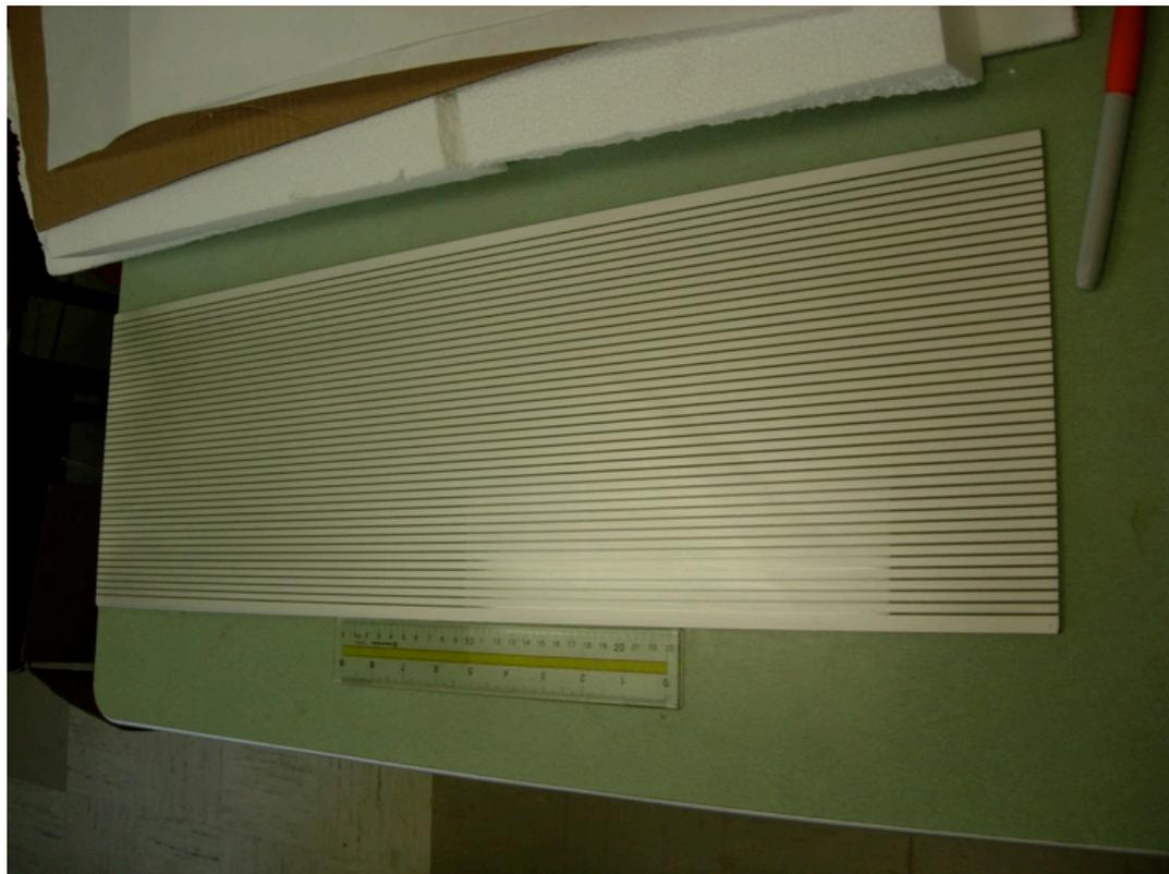
Differential readout at either end allows tiling of MCPs onto supermodule board
