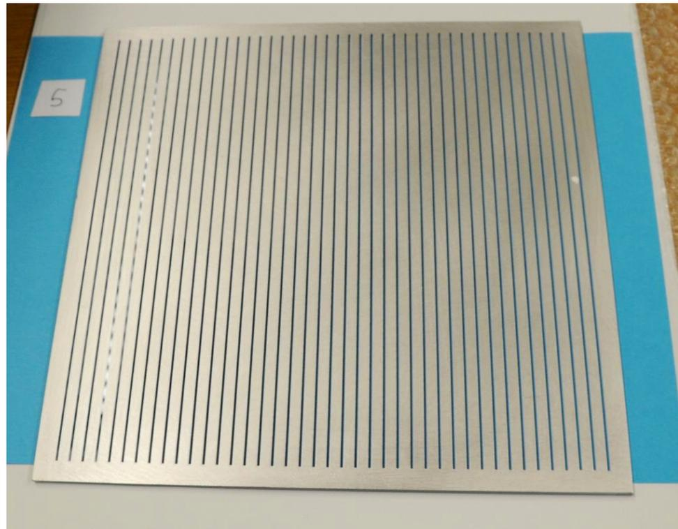
Silk-screen printing of anode ground plane on B33 glass
