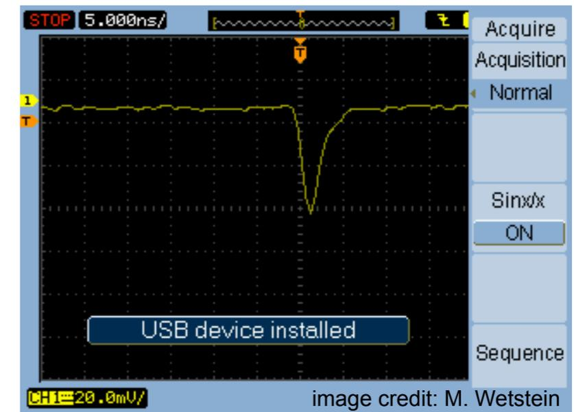
Signal from MCP pair coated with new resistive layer + Al<sub>2</sub>O<sub>3</sub> emissive layer
