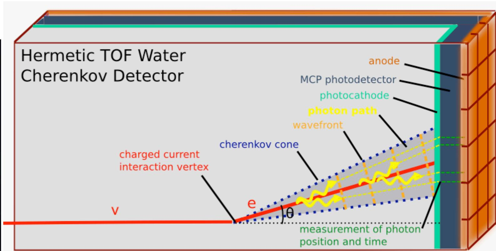
Water Cherenkov neutrino detector (DUSEL) ~80-90% coverage and 3-d photon vertex reconstruction
