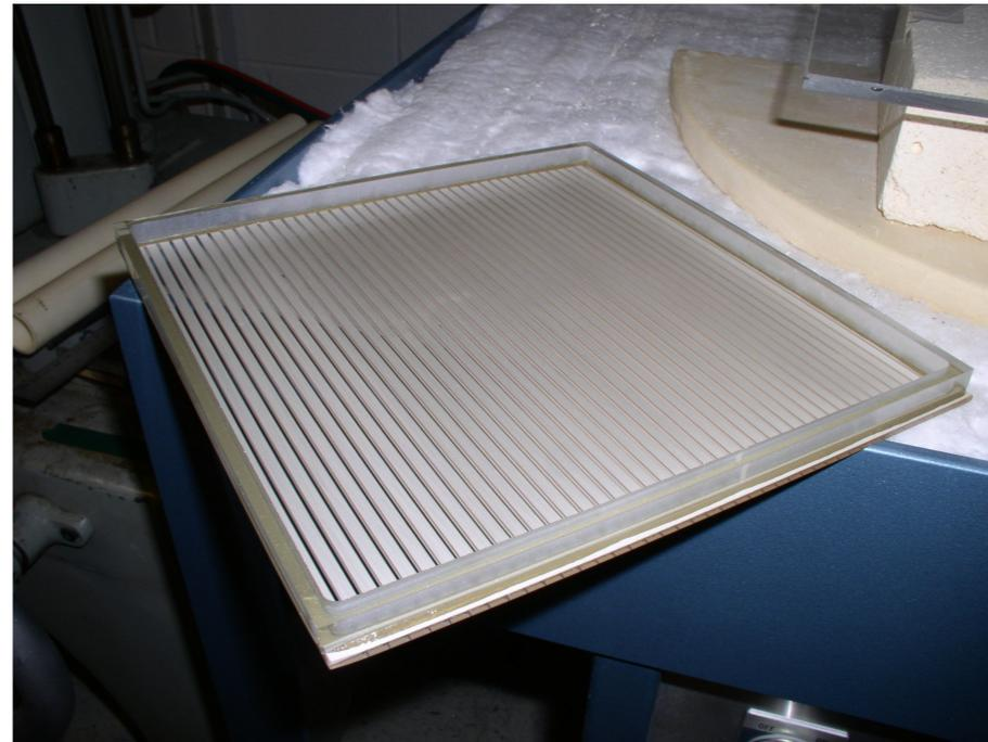
Sidewall bonded to bottom plate with glass frit
