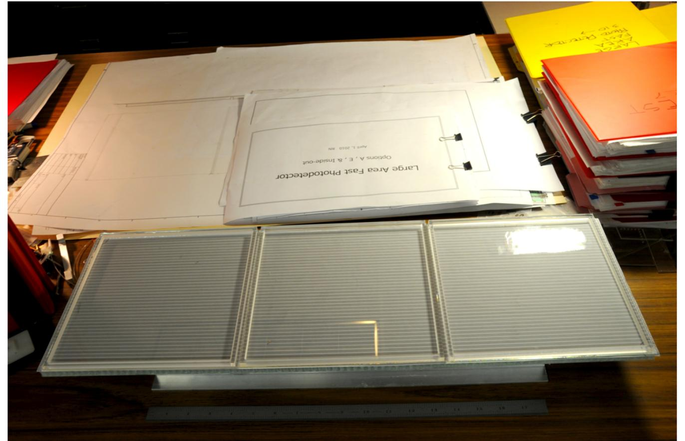
Mockup of three tile supermodule
