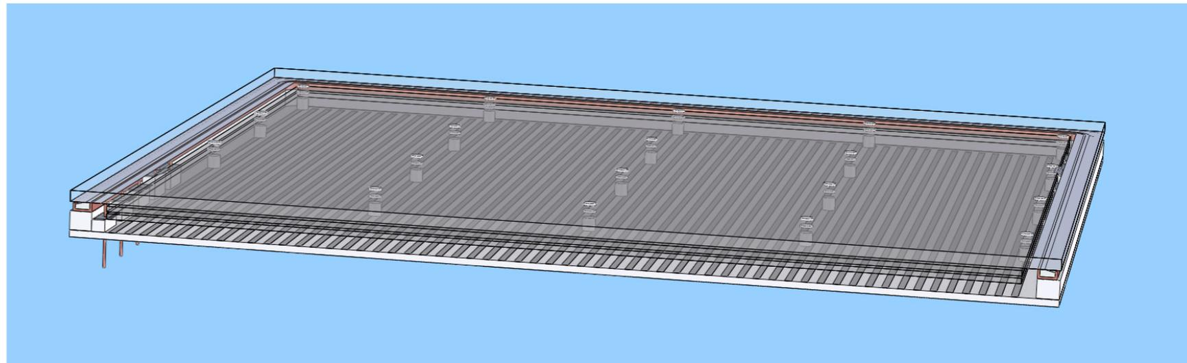
Final assembly with MCP, photocathode
