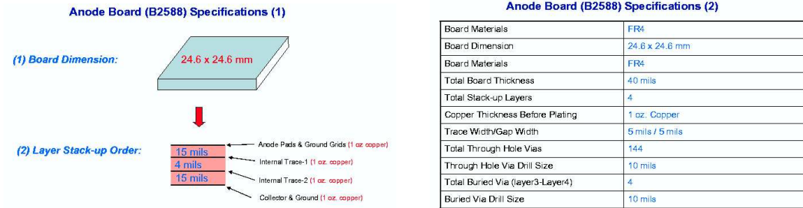
Figure 4: Left: The layers of the anode PC board. Right: A table of parameters for the construction of the first version of the anode prototype.
