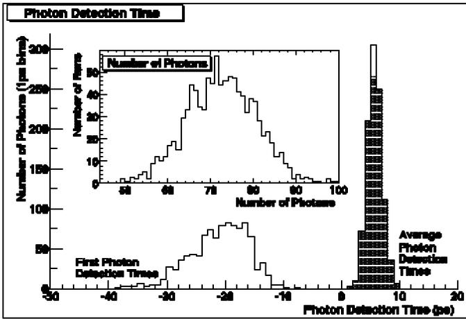
Fig. 6. The spread in first photon detection times and average photon detections times for a set of 1000 simulations of Hamamatsu’s R3809U-58. Inset is the number of photoelectrons detected for each of these simulations.
