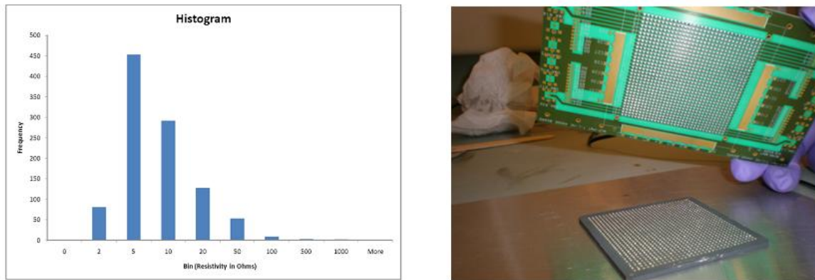
Figure 3: (left) A histogram of the resistivity across the conducting epoxy when attached to a Transmission line board and dummy MCP anode. (right) An image of the actual transmission line board and dummy MCP anode just before being epoxied together.
