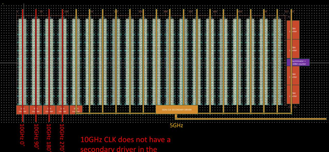
10GHz CLK does not have a secondary driver in the current design!
