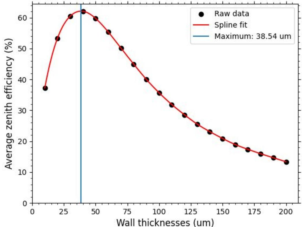
Geant4 simulation of 2.54-cm (1-in) thick NIST lead glass LMCP with 50- $\mu\text{m}$  wide square pore
