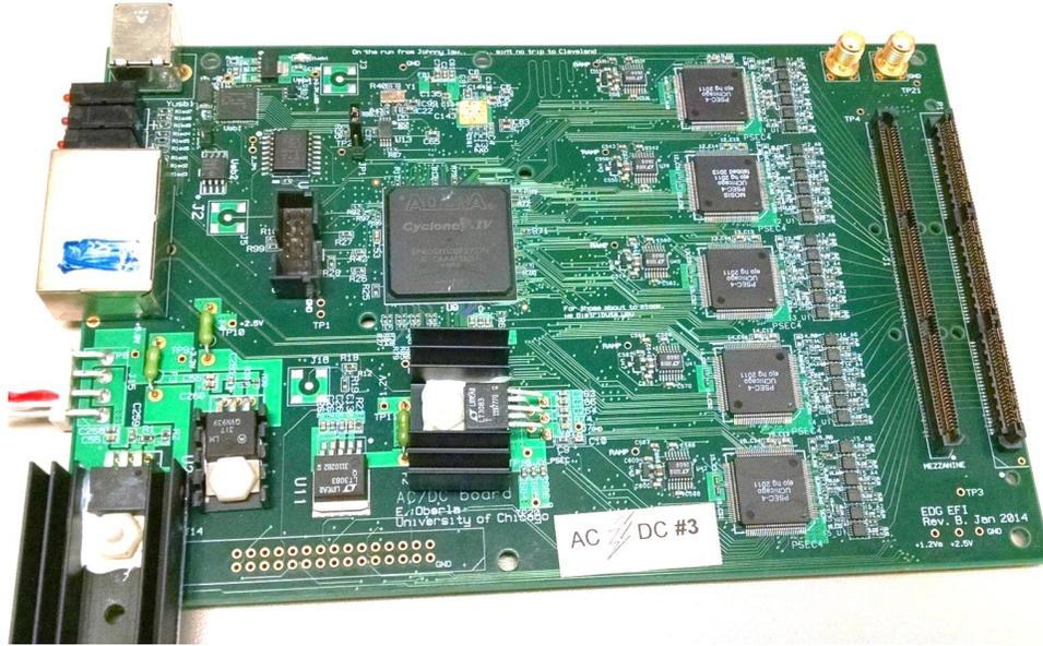
Figure 2.7: The OTPC front-end: the ACquisition and Digitization with pseC4 (ACDC) card. The ACDC card is a 30-channel waveform digitizing board using the waveform-recording PSEC4 ASICs running at a sampling rate of 10.24 GSPS. A 1 GHz 20 dB voltage amplifier card is plugged in the mezzanine slot and the MCP-PMT signal is plugged into the board-to-board slot furthest on the right.
