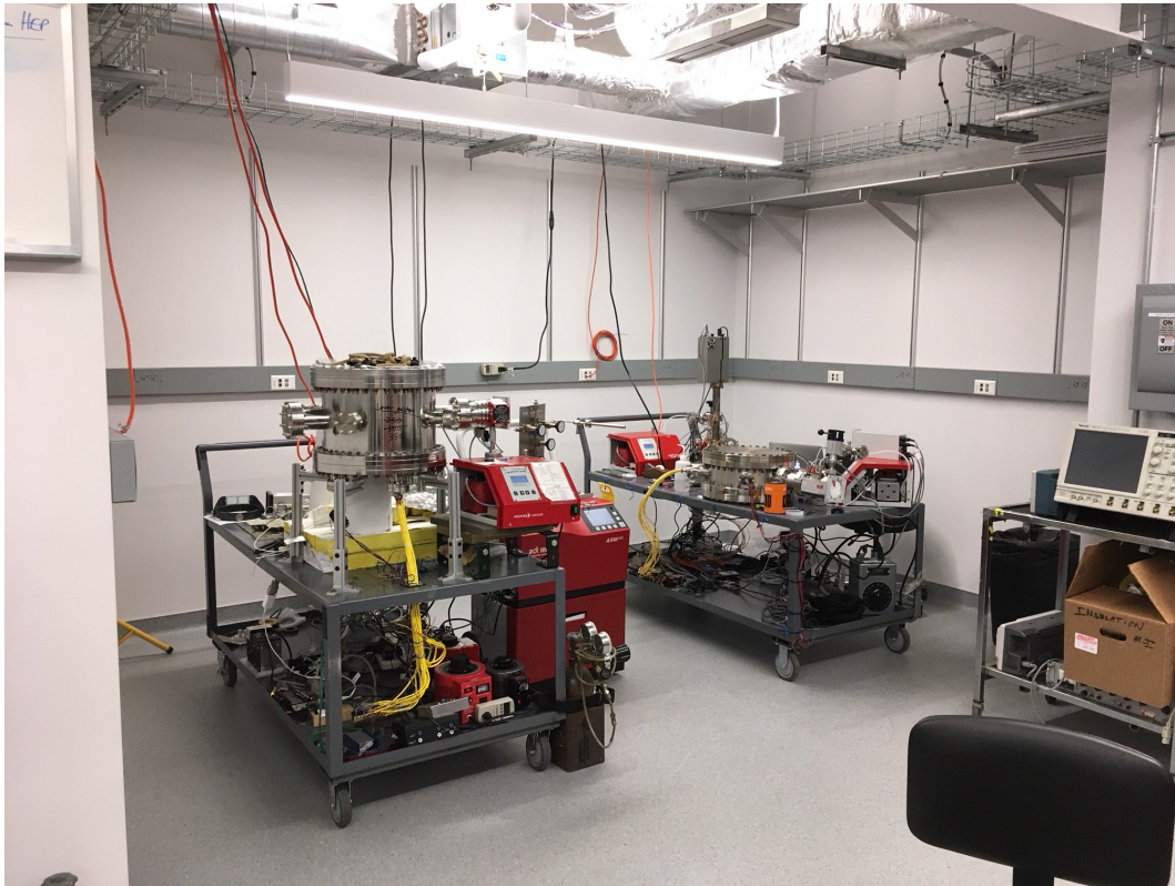
Figure 6: The two Margherita single-tile fabrication prototypes for batch production [9, 10]. With C. Ertley of Southwest Research Institutes we are developing a design of 6 stacks of 3 LAPPDs each per cart, with a 1 week cycle. Six carts would produce 100 tiles per week.
