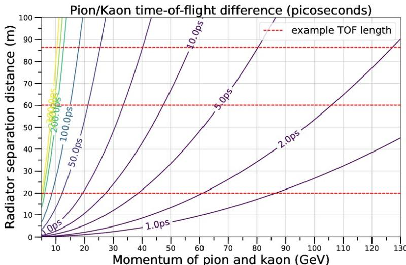
Figure 1: The contours of  $\pi - K$  TOF differences as a function of momentum and the separation of the 2 TOF detector stations in the TB (Evan Angelico [4])
