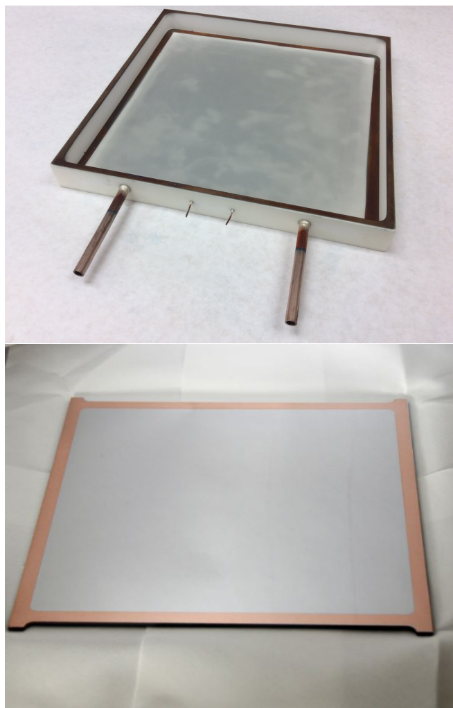
FIG. 4. Top: A two-pin ceramic tile body with metalized sealing surface and NiCr capacitively-coupled anode; Bottom: An entrance window with metalized sealing surface.
