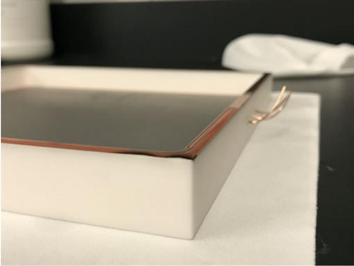
Figure D.4: A sealing metalization being pre-conditioned with a short soak in acetic acid.
