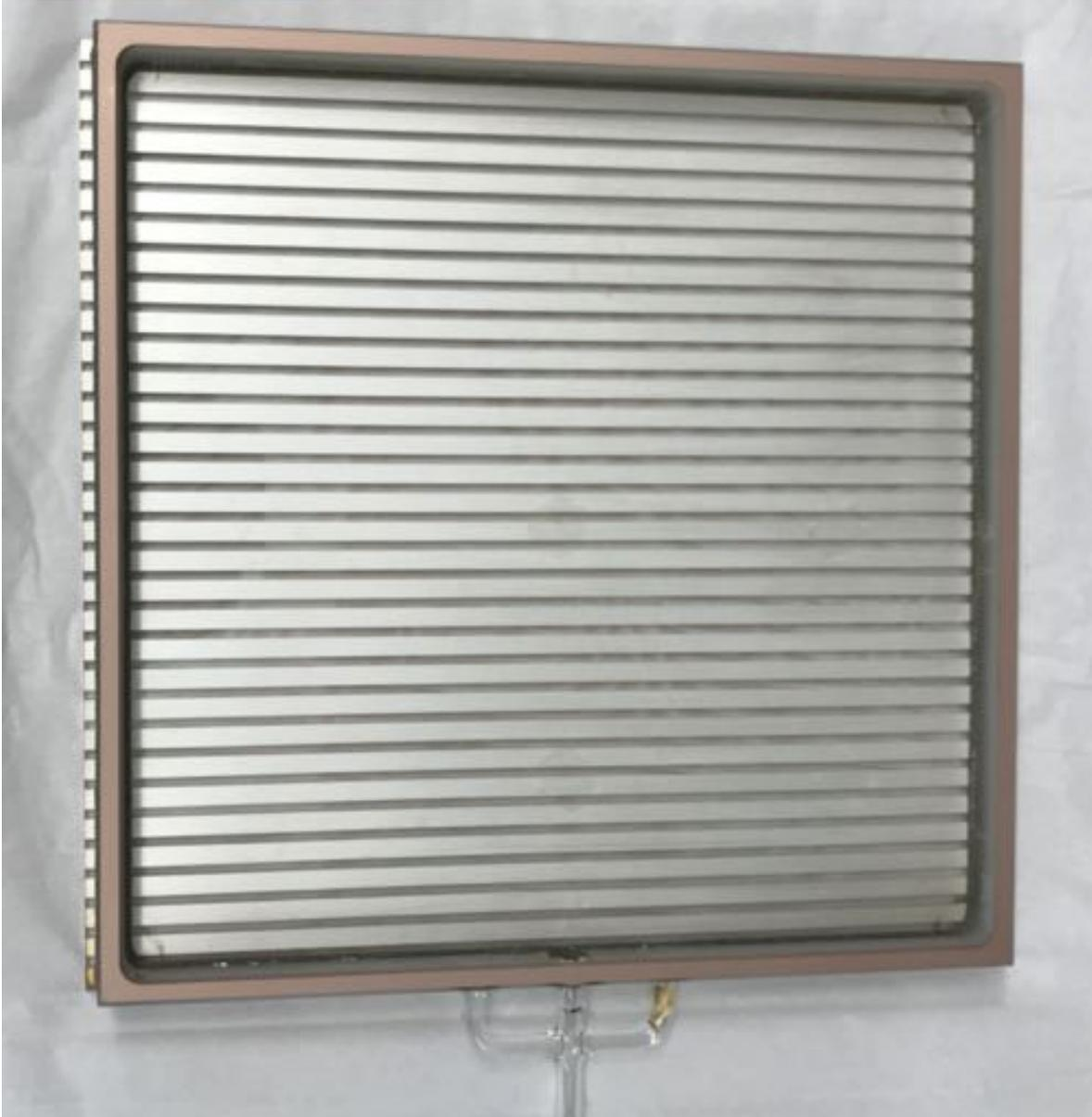
Figure 3.1: Photograph of a strip-line pickup geometry. This pickup pattern was designed and characterized by the authors of Reference [74]. The perimeter is a top-down view of the sealing surface. Each strip has  $50 \Omega$  characteristic impedance when a ground-plane is attached to the air-side of the glass substrate.
