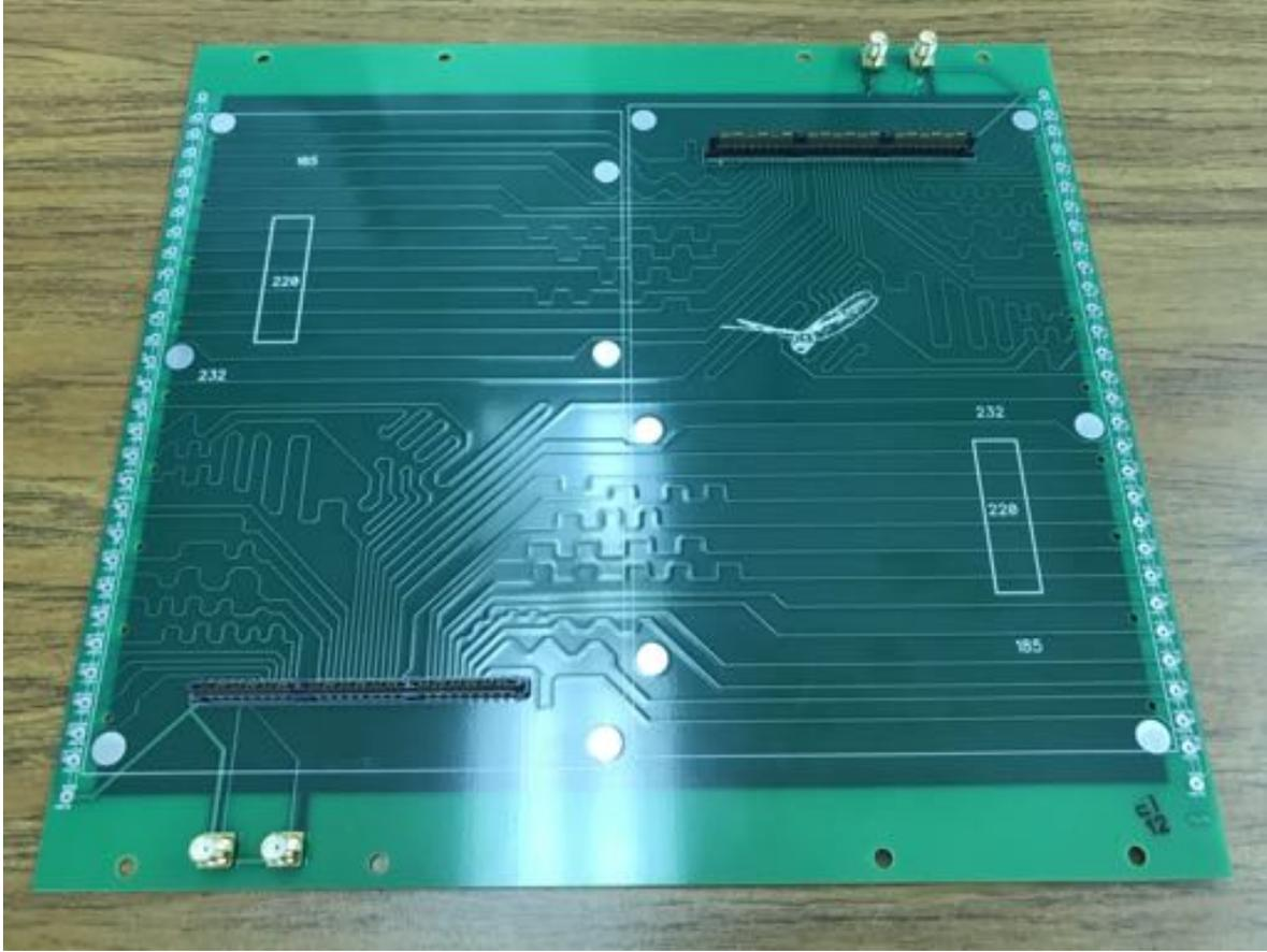
Figure 3.6: Photograph of the ANNIE Analog Pickup Board designed by Bernhard Adams at Incom Inc. Trace lengths are matched to a tolerance of 0.2 mm. Pogo pin contacts, and 10 k $\Omega$  drainage resistors mounted on the surface, can be seen on the left and right sides of the board. Mounting holes that allow for pogo-board compression are seen nearby the pogo pin electrical contacts.
