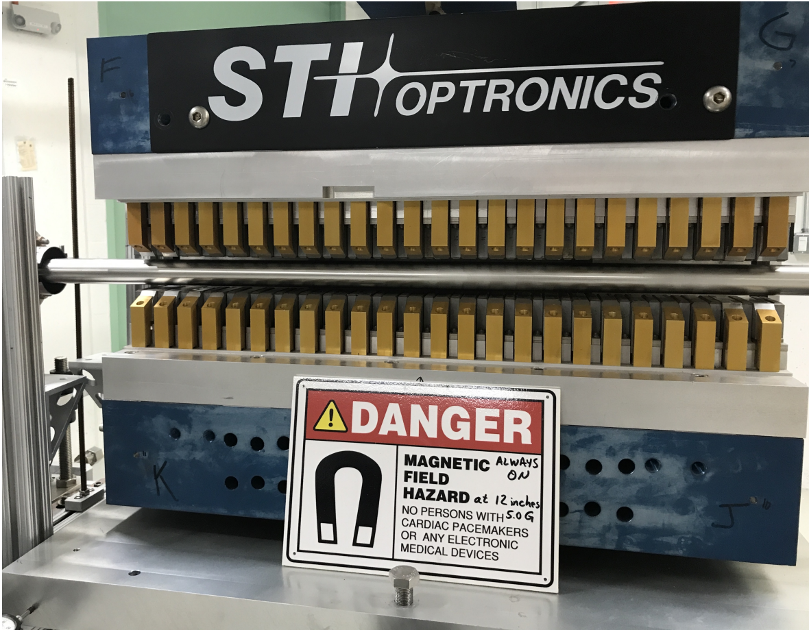
FIG. 1. The SLAC STI Optronics undulator installed in IOTA. This undulator has a K parameter of 1.0 and 10 periods at 55 mm wavelength (see Reference [17]).
