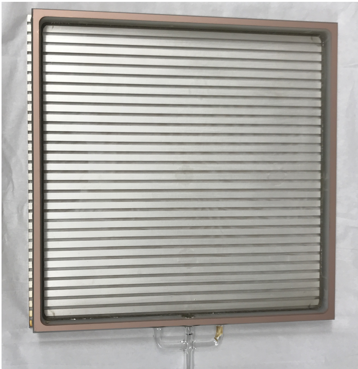
FIG. 11. Photograph of the strip-line anode geometry. The anode was designed to optimize on timing resolution, spatial resolution, and low channel count. Typical spatial resolutions achieved for this 30-channel readout are 1 mm in both dimensions [2]. Typical timing resolutions for single photoelectrons are 50-70 ps.
