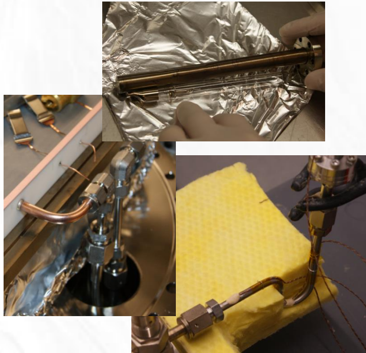
Precision welding of vacuum components for Cs source
