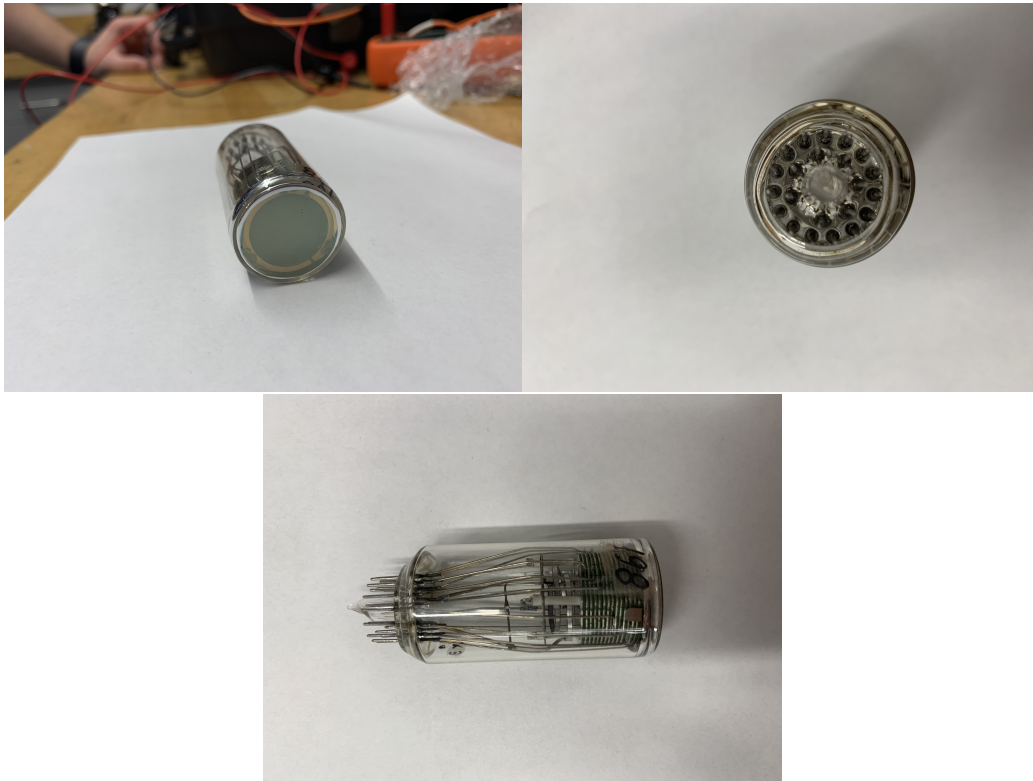
Figure 5: The figure on the upper-left corner is the window of FEU-527 cathode-to-anode photo-multiplier tube. It admits light, while a layer of photo-cathode inside emits electrons. The figure on the upper-right is the base of FEU-527. It has two rows, twenty-two connector pins. The figure on the bottom is the side of FEU-527.
