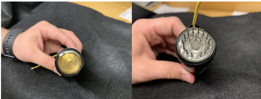
Figure 2: The figure on the left is the window of the cathode-to-anode photo-multiplier tube. It admits light, while a layer of photo-cathode inside emits electrons. The figure on the right is the base of the photo-multiplier tube. It has fourteen connector pins.
