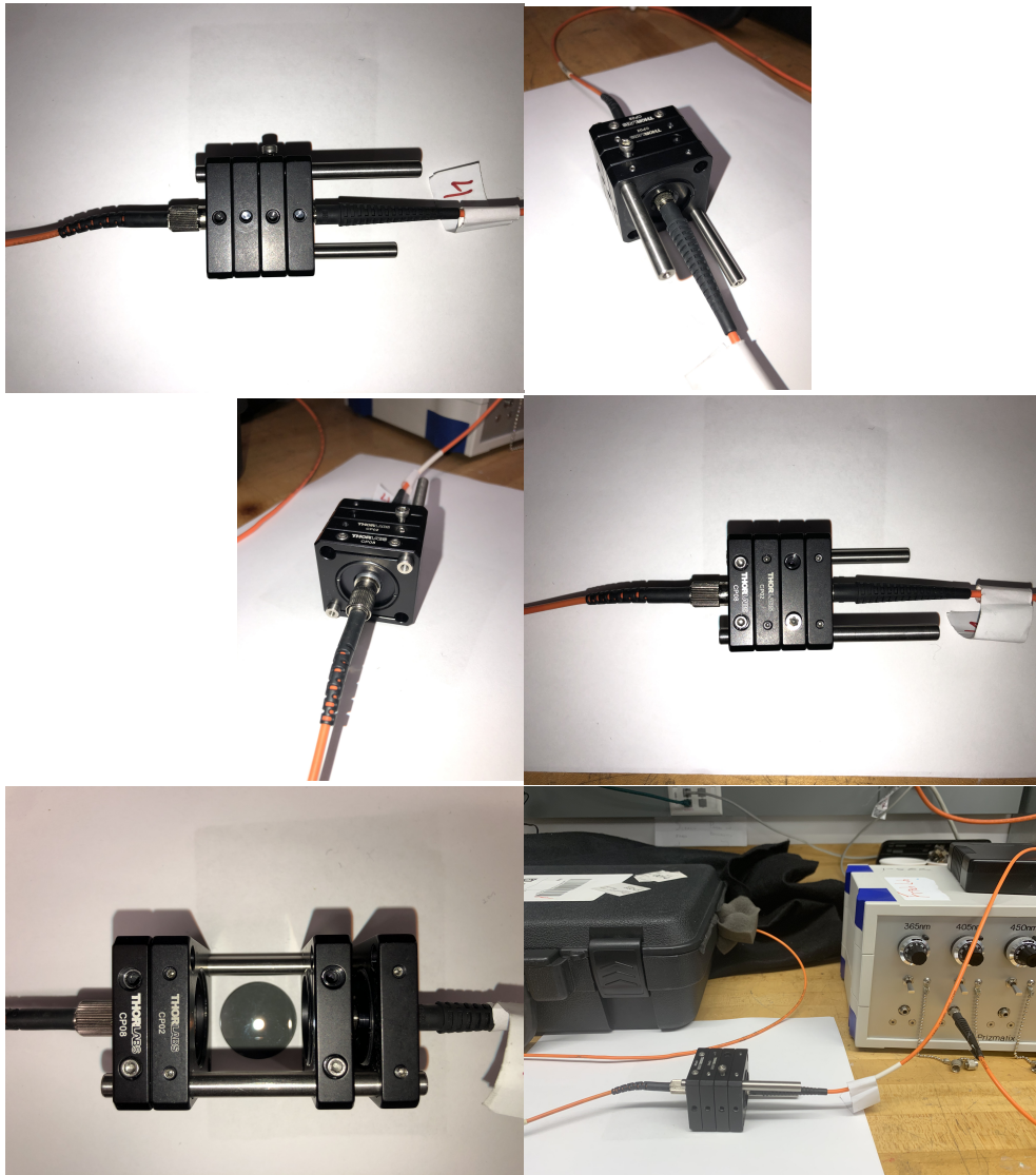
Figure 7: Set-up for adding a filter in the path of the optical cables without opening the dark box. Clockwise from top left: top view, front view, side view, full set-up, expanded view that shows where the filter is placed, and back view. The orange optical cable connects one of the channels of the Prizmatix to the set of four cage plates. The two cage plates in the middle are used for adding filters, while the two cage plates on the side are used to fix the ends of the optical cables. The other optical cable connects the set of cage plates into the dark box, with the end pointing at the window of the photo-multiplier.
