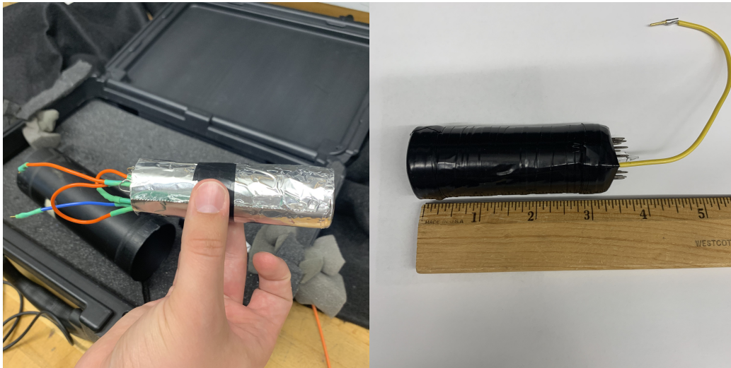
Figure 4: An aluminum guard cylinder is wrapped around the tube, keeping the current running inside the tube, not leaking to the nearby glass. Black tape is wrapped up outside the guard cylinder to insulate the photomultiplier tube from the magnetic shield. A yellow wire is attached to the guard cylinder, which would then be connected to the photo-cathode.
