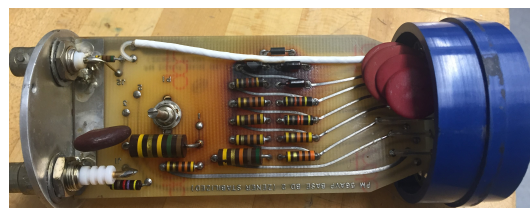
Figure 8: Circuit for Photomultiplier Tube
