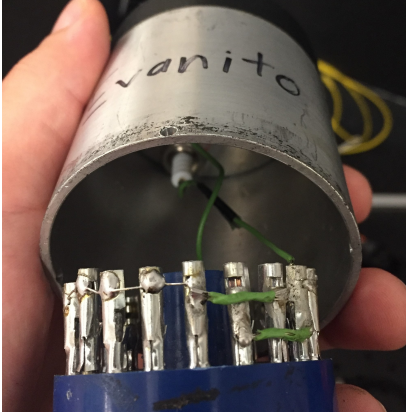
Figure 9: Modified PMT pins
