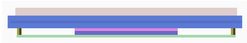
Figure 6: A demonstration of the idea of a plug adapter to connect the capacitated leads on top of the tile directly to the board(s) underneath. Dark blue represents the adapter. Pink and purple represent the male and female ends of the ribbon cable that fit together.
