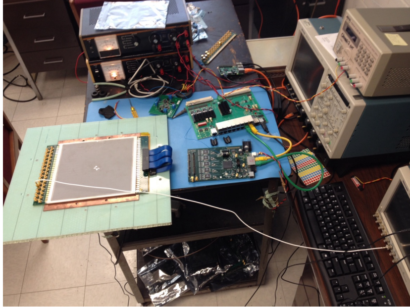
Figure 13: The test setup. The PSEC chips are powered by the A4490, a signal from the AWG is fed to a single PSEC channel, and data is collected via the Raspberry Pi.
