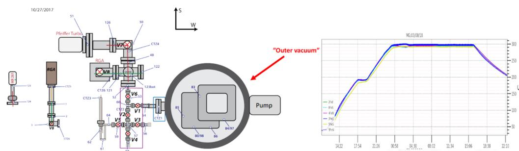
(Left:) Schematic view of the processing system that includes the dual-vacuum system and alkali transport system. (Right:) Typical bake-out and indium seal heat cycle.
