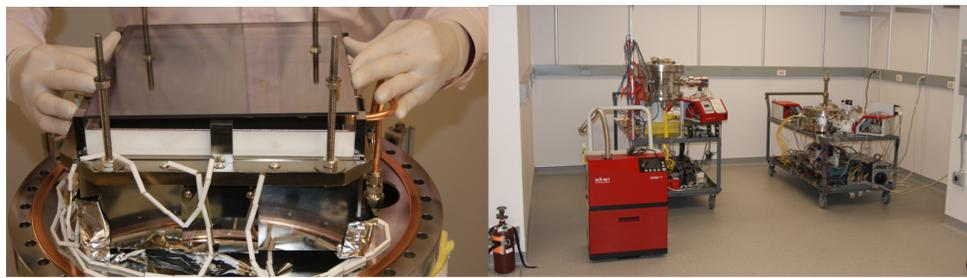
(Left:) Air-transfer of the window with pre-deposited layer of Sb. (Right:) University of Chicago PSEC Lab with two vacuum processing chambers. Due to their compact size, potentially many chambers could be operated at the same time at a future LAPPD production facility, using a shared vacuum distribution system. Each vacuum processing chamber could accommodate several LAPPDs. This batch production strategy would be similar to PMT batch production.
