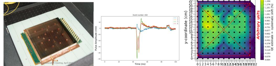
(Left:) Complete Gen-II LAPPD tile-21. (Middle:) Pulses from tile-21. (Right:) Final photo-sensitivity map of the tile-21 in arbitrary units. Tile-21 was an early test of cesium transport. Improved photo-cathode uniformity is expected in future devices.
