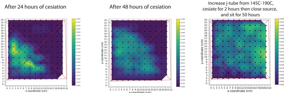
In-situ photo-cathode synthesis showing photo-sensitivity expressed in arbitrary units. Direct measurement of photo-current and absolute QE were precluded since the photo-cathode, MCPs, and the anode were interconnected with an internal high-voltage divider as part of a simplified strategy to power the tile (see Refs. 2-3). Future devices will allow direct measurement of photo-current and calibrated QE.
