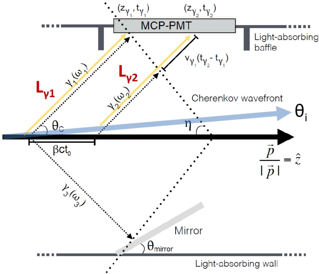
The time projection of the direct Cherenkov photons on the OTPC z-axis is a measure of the Cherenkov angle ( $\beta$ ) and the particle angle with respect to the OTPC longitudinal axis
