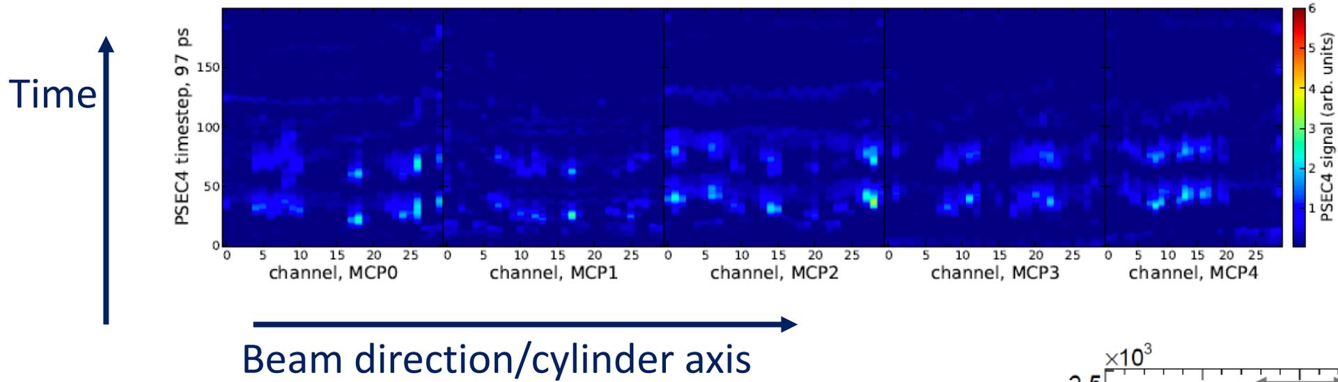
Observe ~770 ps timing separation corresponding to (diameter)/(group velocity)
