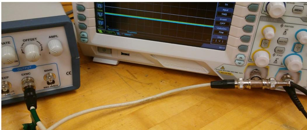
Figure 7: Connections at the Function Generator on the left and Oscilloscope on the right.
