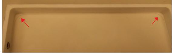
Figure 5: Rim on ceramic base Coorstek base 1 inner surface.
