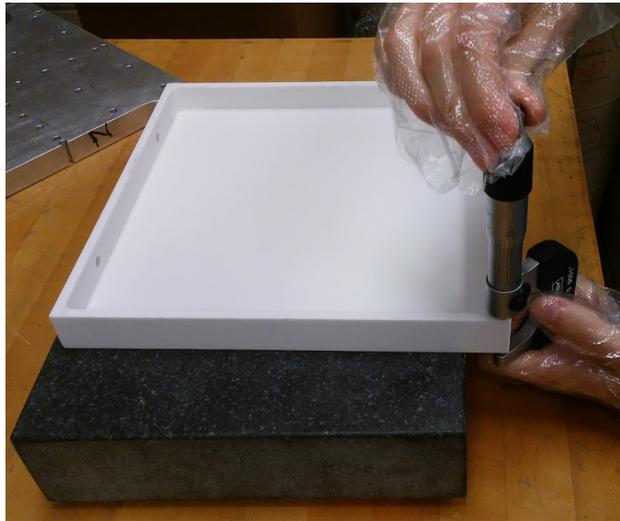
Figure 2: Measurement of the height at 8 points of the ceramic base using a micrometer.
