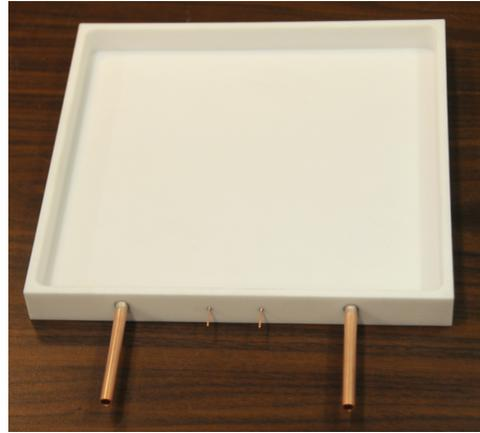
Figure 1: Ceramic base measured and characterized for quality control (for a ceramic base spec sheet with dimensions and tolerances see Appendix A)[2].
