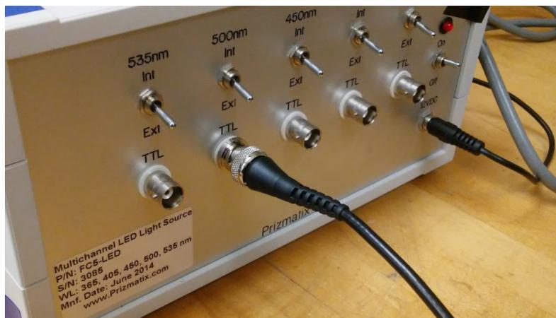
Figure 6: Connections at the back of the LED Box.
