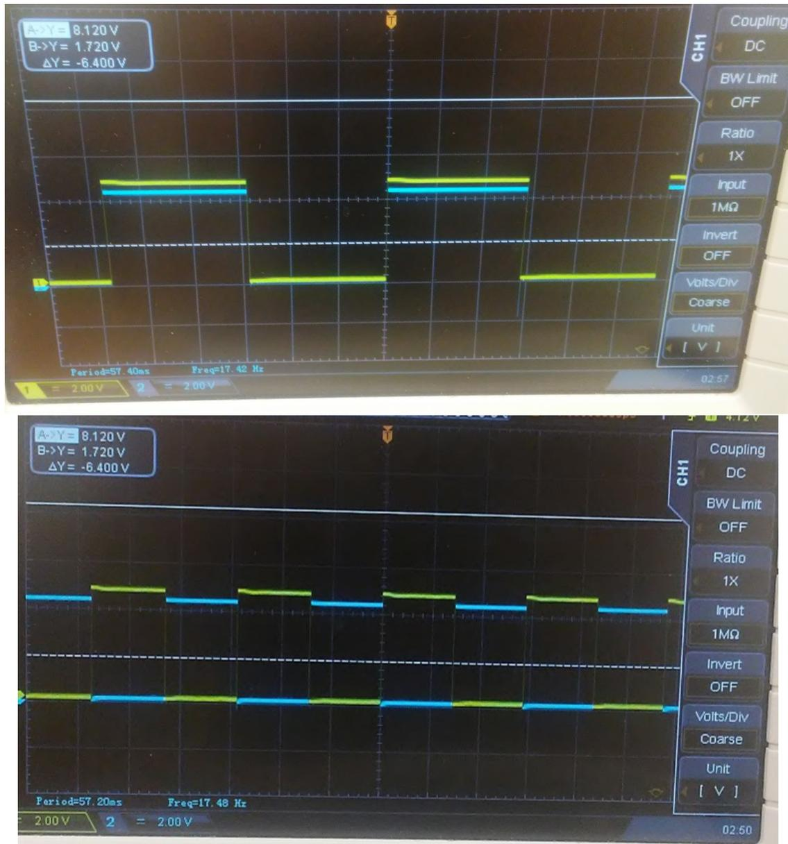
Figure 8: Top: In-phase oscilloscope display of signal. Bottom: Out-of-phase oscilloscope display of signal. Yellow: display of the reference TTL signal from function generator. Blue: display of the TTL signal from the Differential circuit. The Blue has a slightly lower amplitude after passing through the circuit at  $\approx 4V$
