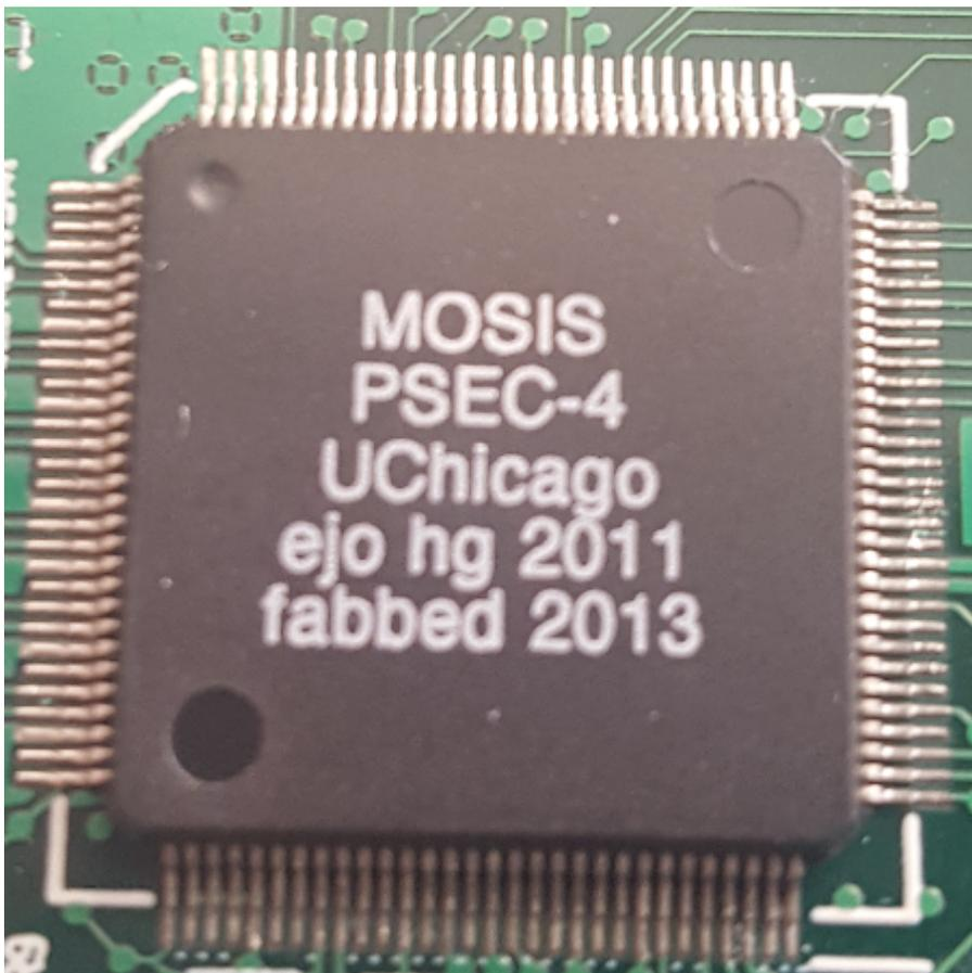
Figure 2: A close up view of the PSEC4 chip, the ADC used in the DAQ.
