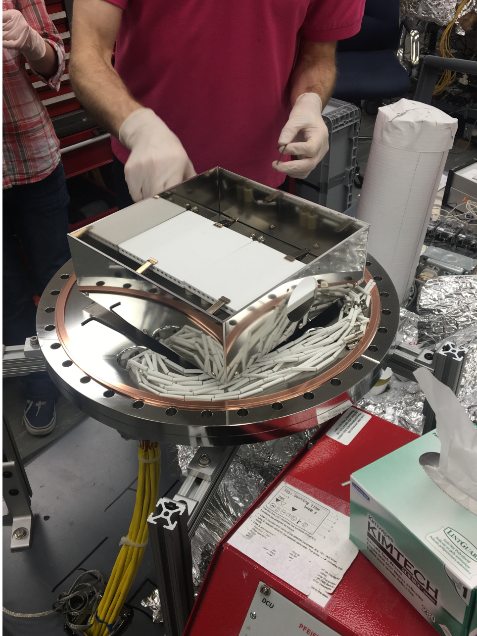
Figure 6: The fixture contains two white Ni-chrome heaters at its lowest level. Since these heaters operate in ultra-high vacuum, they are largely radiative. Thus, stainless steel foil acts as a reflective insulation. Ten thermocouples monitor the internal temperature.
