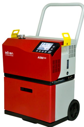
Figure 9: Helium leak detector (ASM340), which was used to pump out the Margherita 2 Outer Manifold in conjunction with the Turbo Pump. While helium was sprayed into the CF and Swagelok leak-checking ports, the leak detector readings, in mbar*L/s He, was monitored for increase. A peak in He flow rate indicates that a leak has been momentarily sprayed; a plateau indicates that a leak has been sprayed for an extended period of time.
