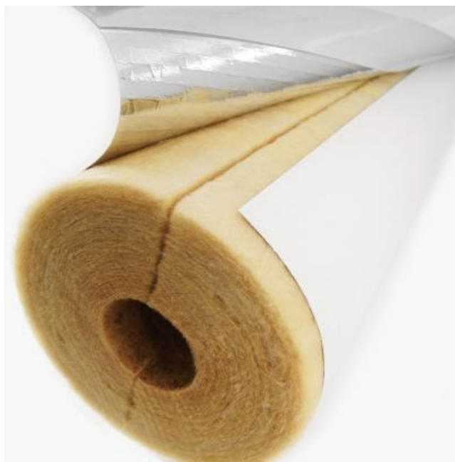
Figure 12: Fiberglass piping used to construct a thermal insulation system for the large tube manifold. When fiberglass is handled, skin should be covered and respiratory precautions should be taken. Suction clean the work area once fiberglass insulation has been installed.
