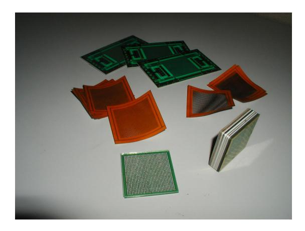
While Indium Solder was being explored to join the MCP to a read out PC Board we contacted Best to provide us with Kapton Laser drilled Masks to experiment this assembly method.
