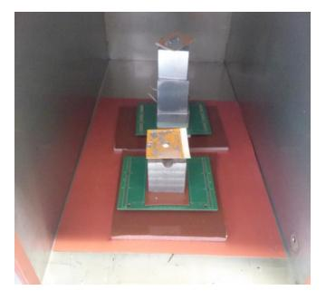
Large sheet of High Temperature Silicon Rubber again is used at base of curing oven which the individual aluminum plates used to transfer assemblies into the cure oven.
