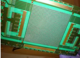
PC Board fabricated to read out each 4096 channels. This board has In Solder applied to each pad. Surface was roughed up with 3M Scotch and cleaned in previous detail.
