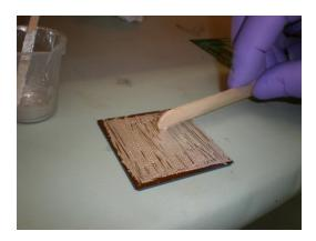
With 4096 Pad Kapton aligned over a Burle MCP electrical Back Plane. Ag Epoxy is weighed out and placed on assembly. During course of discovering true amount of Ag Epoxy is needed, a cup was used and reweighed to trim down bulk to a more conservative mix, for future applications.
