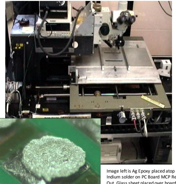
Indium solder on PC Board MCP Read Out. Glass sheet placed over board compresses Ag Epoxy to replicate a MCP placement.
