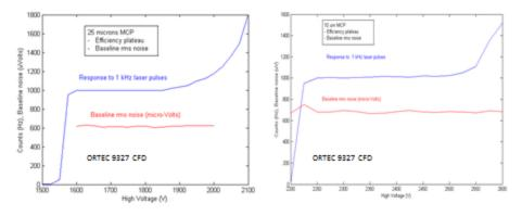
Efficiency plateau and baseline noise (left: 25 μm, right 10 μm) Plateaux are 300V wide for both MCPs Baseline rms below 1 mV rms (system noise), no dependence with the High Voltage
