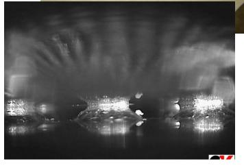
Ag/In Solder pad check with microscope on edge view.
