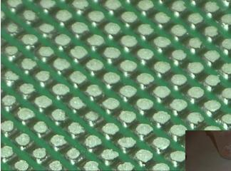
PC Board with glass placed over Ag Epoxy to reproduce pressure excreted by a MCP during cure cycle. This sampling was inspected for over flow and consistency of volume uniformity, during application of un-cured epoxy.
