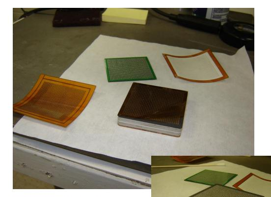
A mechanical grade MCP was obtained along with a simple 4096 Pad PC Board to be used to test weight application during oven cure.
