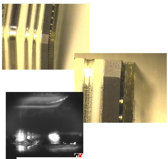
Edge view inspection can only penetrate a few rows of pads. But unlike a 2D X-Ray image does not show form of individual columns of Ag Epoxy.
