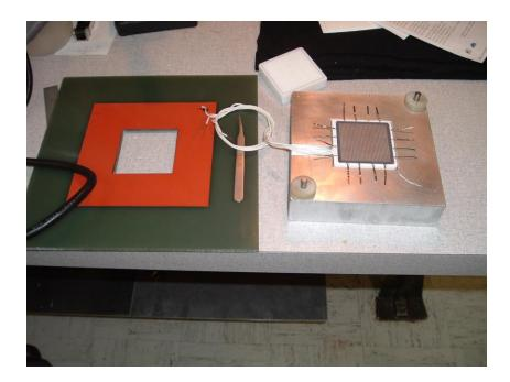
The heat sink used for this was an aluminum block with a pocket milled into it to 'nest' the MCP during this procedure.
