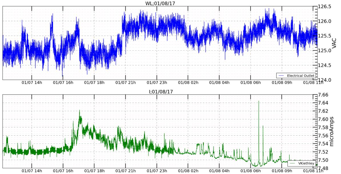
Figure 5: The Keithley is a measurement of the current across all the MCPs in the Margherita. This figure juxtaposes Wall Voltage RMS with Keithley measurements. Although it is impossible to account for other factors, the two measurements exhibit independence and no strong correlation (Fig 6). Kiethley, thus, has historically displayed independence of its power supply.
