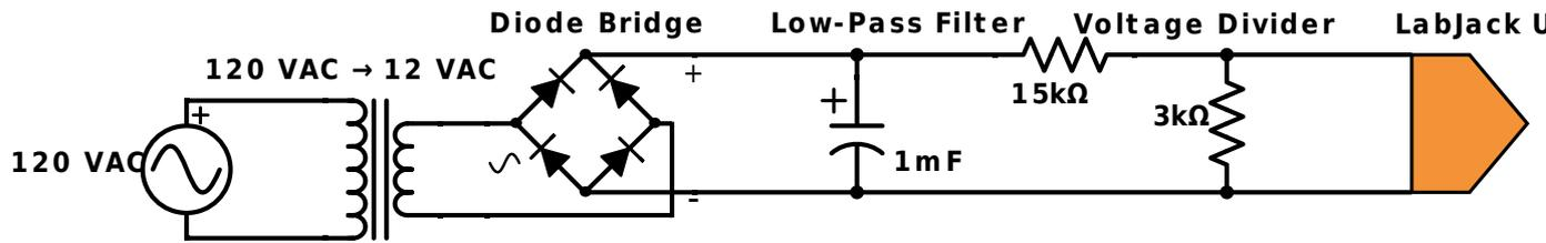
Figure 1: Wall Voltage Monitor Schematic. 120 VAC wall supply is initially stepped down to 12 VAC. It is then rectified by a diode bridge and low pass filtered to smooth the resulting DC signal. Finally, this DC signal passes through a voltage divider to reach a final value that the LabJack U6 can read. A Raspberry Pi converts this DC voltage to the corresponding AC voltage.
