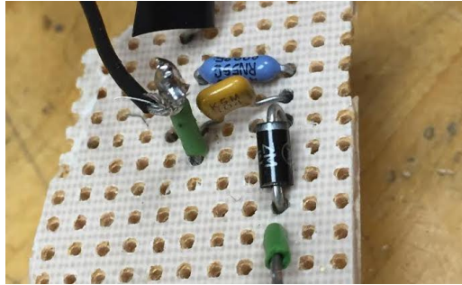
Figure 2: Photo of an early rendition of the circuit we used for the sound monitor. The soldering is not clean, as this was a first attempt at soldering.
