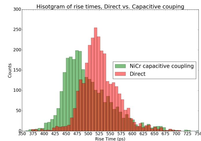
Figure 4: The capacitive readout scheme preserves rise-time of pulses (rise time is a key factor in timing resolution)
