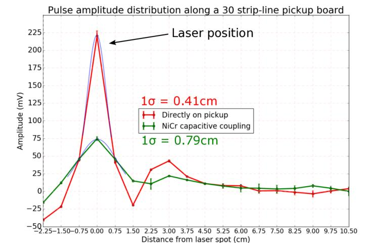
Figure 5: Each strip-line pickup has an associated amplitude. Strips far away from the laser spot have lower amplitude. The capacitive anode spreads the amplitude distribution in space.
