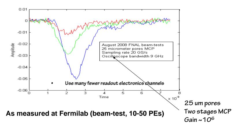
$I(1PE) = dQ/dt \sim 1.6 \times 10^{-19} \times 5 \times 10^{5} / 250 \text{ ps} = 320 \text{ uA}$ Expect:  $16 \text{ mV} @ 50 \Omega$
