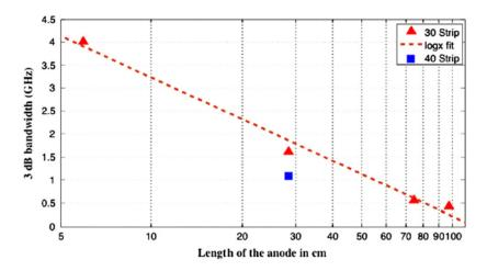
The 0-tile anode (left-most data point) has a 3dB bandwidth of 4.1GHz. I found the 0-tile anode that was used to produce the result, and also made a new one. The results for measuring these two tiles are:
