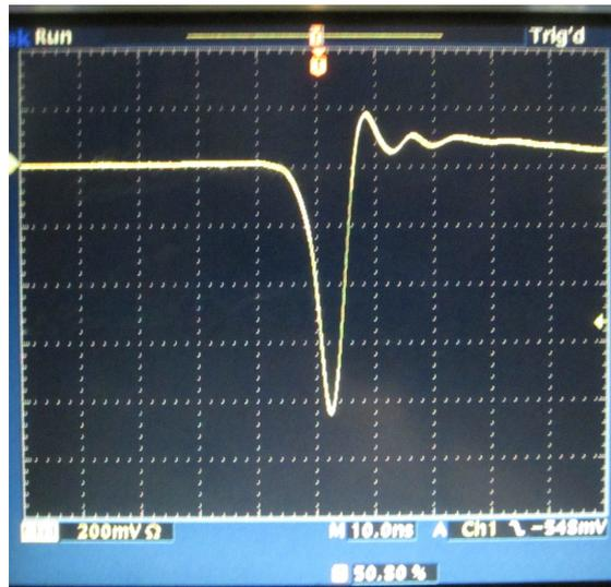
**Figure 8.** Average single event pulse shape for a 20 cm, MCP pair, 20  $\mu\text{m}$  pore, 60:1 L/D, ALD MCPs.
