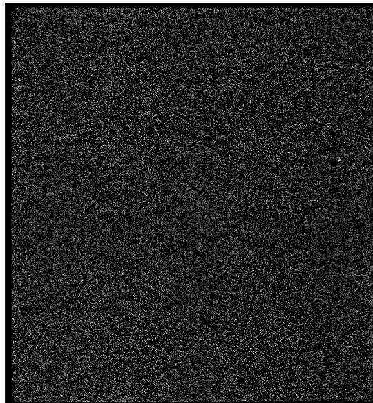
**Figure 10.** Background event image for a pair of  $20\ \mu\text{m}$  pore, 60:1 L/D, ALD MCPs.  $0.055\ \text{events cm}^{-2}\ \text{sec}^{-1}$ .
