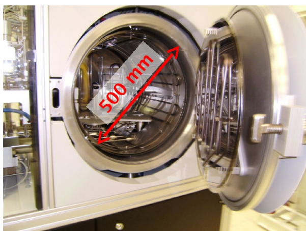
Figure 25. The Beneq Atomic Layer Deposition facility installed in the Energy Systems Division at ANL, used to functionalize the Incom capillary plates with resistive and secondary-emitting layers. The precursor flow path required extensive modification in order to establish uniformity over the 6.5 m 2 surface area of each capillary plate.
