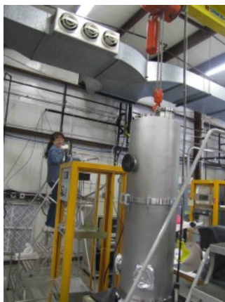
Figure 24. Left: The Fermilab UHV evaporation facility constructed to deposit NiCr electrodes on the top and bottom surfaces of LAPPD TM capillary wafers; Right: A chart of the number of wafers metalized on both sides at the Fermilab evaporation facility versus time.
