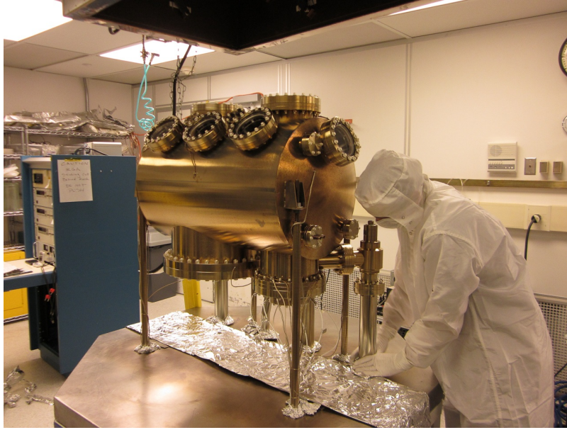
Figure 26. The UHV photocathode and detector assembly facility constructed for LAPPD at the Space Sciences Laboratory, University of California, Berkeley .
