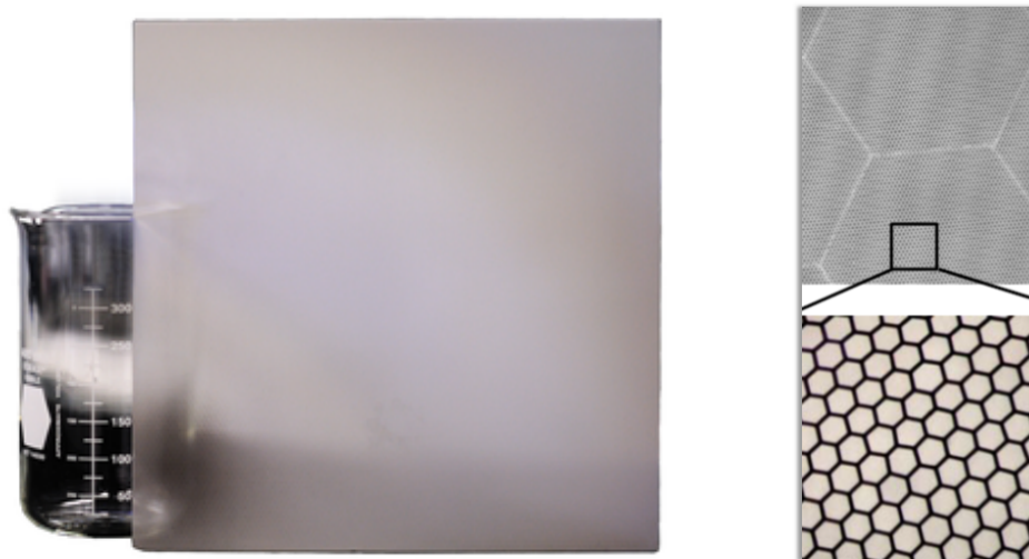
Figure 4. Left: An 8" × 8" glass capillary substrate developed by the Incom corporation. Each substrate contains approximately 80 million 20-micron-diameter capillary pores. The open-area ratio is typically greater than 65%, making the plate appear transparent. Right: A close-up of a similar glass substrate showing the 20-micron capillary structure.
