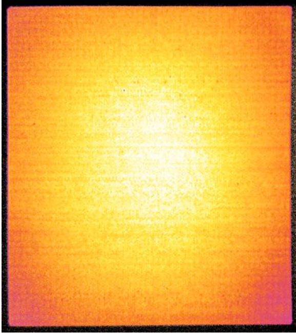
Fig. 18: Gain characteristics for a 20 cm MCP. \text{Al}_2\text{O}_3 ALD 20 \mu\text{m} pore, 60:1 L/d borosilicate MCP. NiCr layer applied to both sides of the MCP pair.
