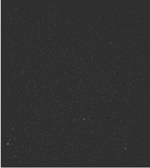
Fig. 21: Background Image. 20 cm square, 8° bias, 60:1 L/d ALD borosilicate MCP pair, Total Rate \sim 0.17 counts \text{cm}^{-2} \text{sec}^{-1} . Rate without hotspots < 0.04 counts \text{cm}^{-2} \text{sec}^{-1}
