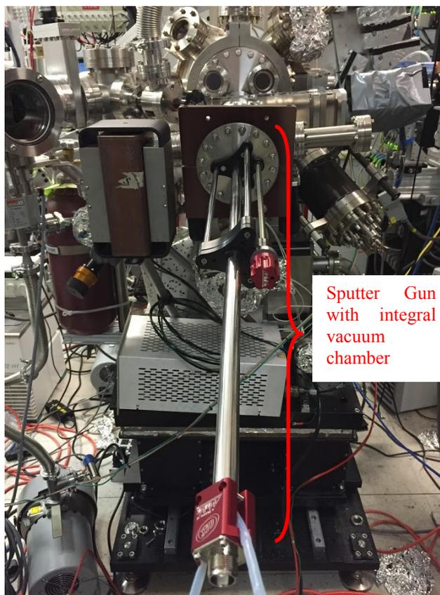
Figure 3: Sputter target mounted on cathode growth and analysis chamber, in G3 line x-ray hut.
