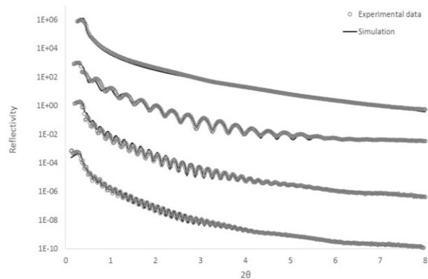
Figure 6: XRR for the substrate (top) and each growth layer (increasing thickness going down on plot), along with the theoretical fits.
