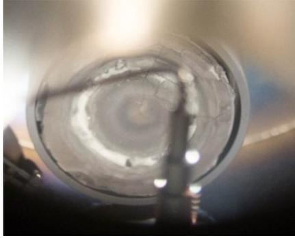
Figure 4: Sputter target after several runs of sputtering.
