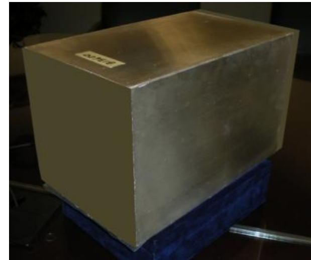
228 mm (9") square capillary block
