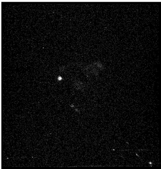
Fig. 18. Background event image accumulation (1000 sec) for a 20 cm, 20  $\mu\text{m}$  pore, 60:1 L/d ALD-MCP pair, 0.7 mm pair gap 400 v, gain  $\sim 1 \times 10^7$ . Overall background 31 events  $\text{sec}^{-1}$  including the observed patches and “warm spots”, resulting an average rate of 0.078 events  $\text{cm}^{-2} \text{sec}^{-1}$ .
