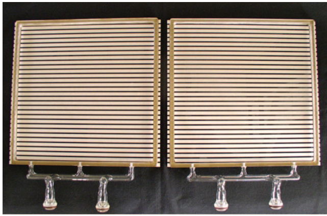
FIG. 16. A pair of demountable tile bases from Joe Gregar (ANL Glass Shop). These consist of a glass side wall fritted onto a 30-strip “frugal” glass anode and are used with an O-ring sealed window to test the MCP-spacer stack of the frugal tile at the APS laser facility. The pump ports are reinforced for mechanical strength.
