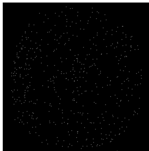
Fig. 7. Image of background event spatial distribution for a back-to-back pair of ALD coated borosilicate MCPs with 20 \mu\text{m} pores, L/D=60:1 , pore bias 8^\circ , 25 mm active area, 1000 s accumulation, 2.5 \times 10^6 gain, 1100 V per MCP. Background rate 0.096\text{events cm}^{-2}\text{s}^{-1} .
