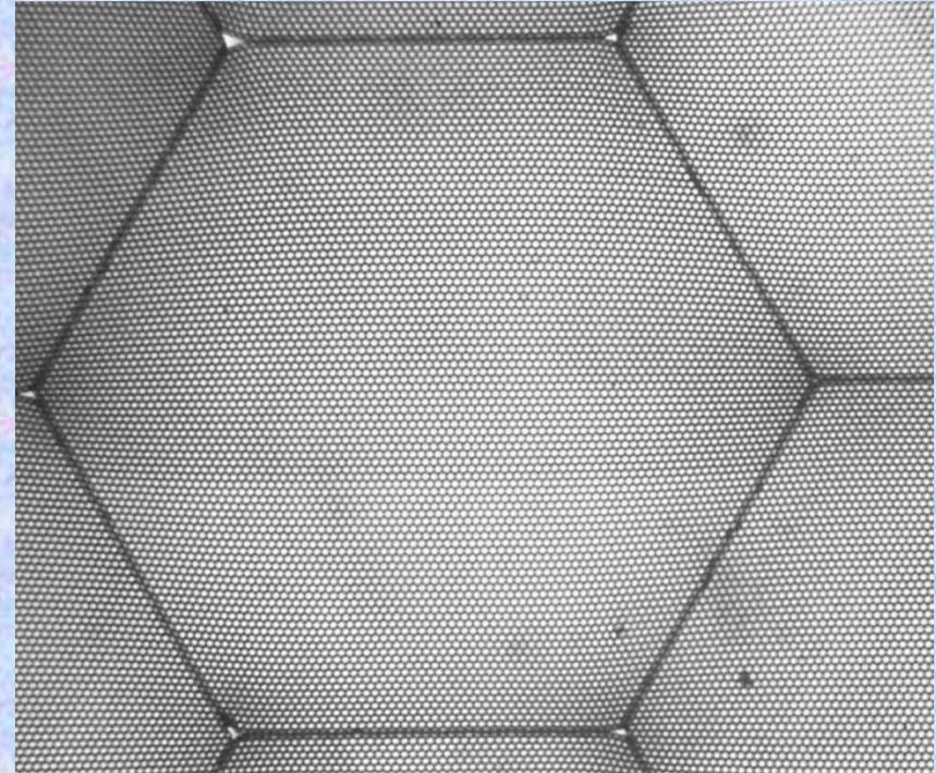
Photo of a  $20\mu\text{m}$  65% OAR,  $8^\circ$  bias, 60:1 L/D, finished substrate, with ALD coating.
