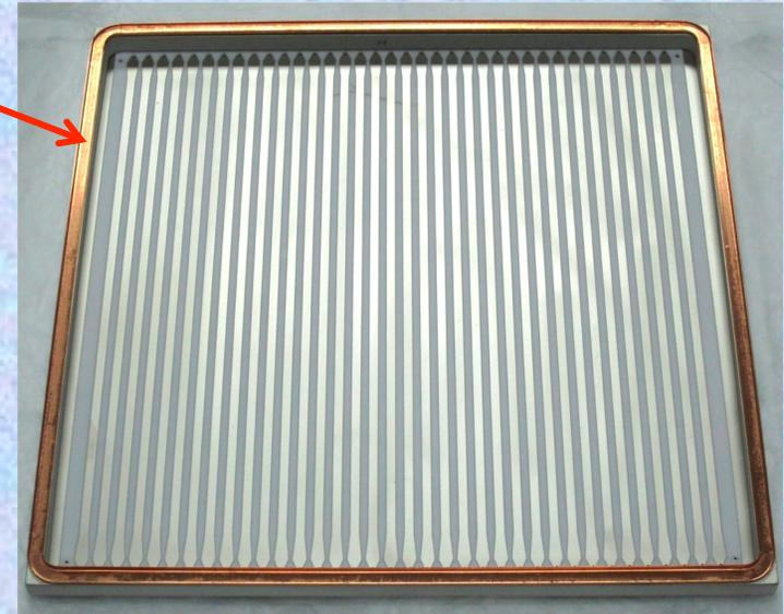
**Ceramic body with Cu Indium well and strip anode.**
