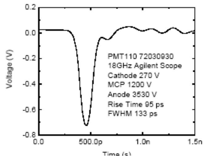
6  $\mu\text{m}$  pore MCP PMT
