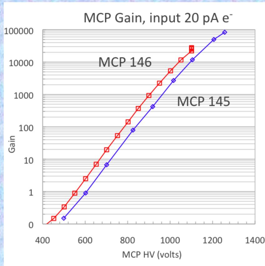
Single MCP tests in DC amplification mode show imaging and gain very similar to conventional MCPs. Sample imaging performance has improved dramatically with substrate and ALD coating process improvements.
