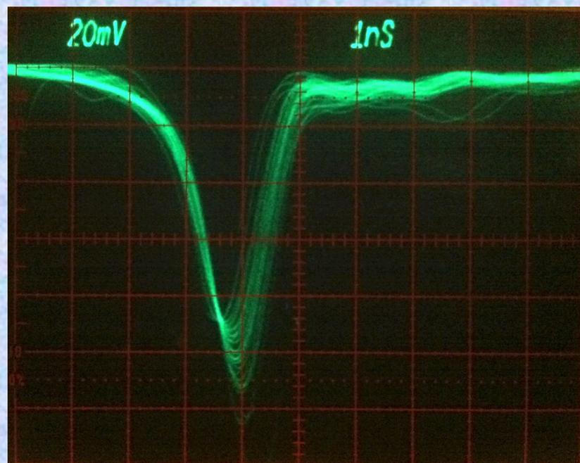
ALD borosilicate MCP pair, 20 $\mu$ m pore, 60:1 L/d, 8 $^\circ$  bias, 0.7mm/1000v MCP gap. Single event pulses are ~1ns wide. ~Typical response for 20 $\mu$ m pore MCPs.
