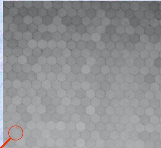
**Visible light transmission for a 20  $\mu\text{m}$  pore 65% open area borosilicate micro-capillary ALD 200 mm MCP. Pore distortions at multifiber boundaries, otherwise very uniform.**
