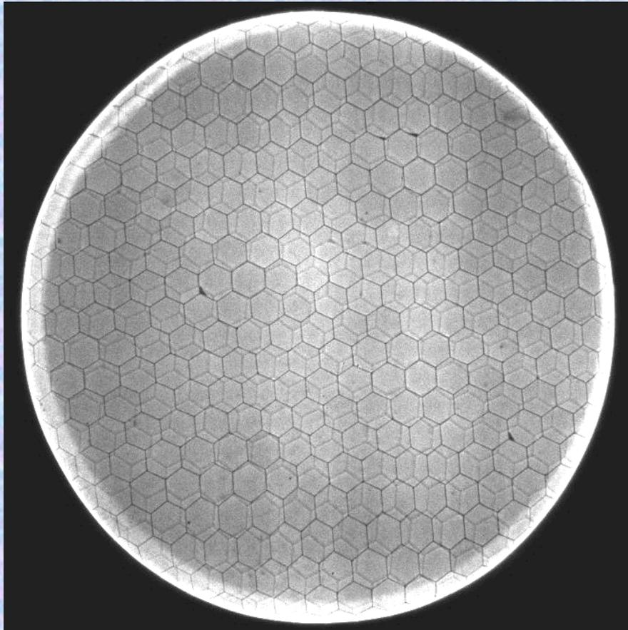
**Image of 185nm UV light, shows top MCP hex modulation (sharp) and faint MCP hexagonal modulation from bottom MCP. A few defects, but generally very good. Edge effects are field fringing due to the MCP support flange.**
