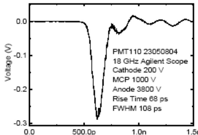
3.2  $\mu\text{m}$  pore MCP PMT
