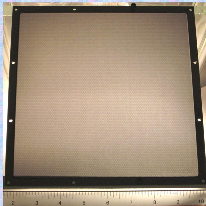
**20cm MCP showing the multifiber stacking arrangement, 40 $\mu\text{m}$  pore,  $8^\circ$  bias.**
