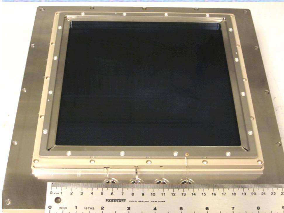
20cm MCP detector showing the cross delay line anode readout. Gives  $< 100\mu\text{m}$  spatial resolution,  $\sim 100\text{ps}$  timing
