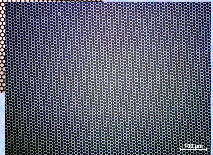
Photo of a 10  $\mu$ m pore, 65% open area borosilicate micro-capillary ALD MCP.
