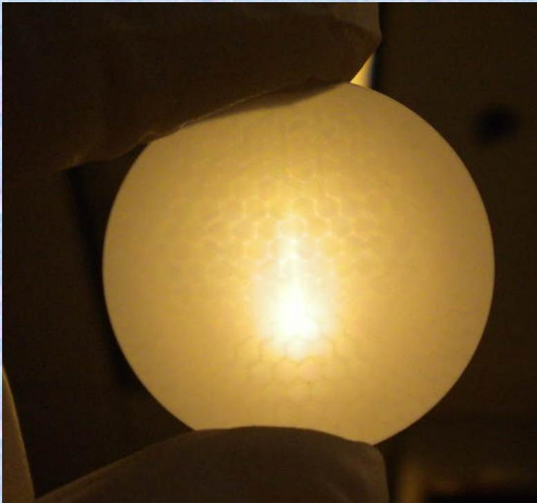
Photo of a  $20\mu\text{m}$  65% OAR,  $8^\circ$  bias, 60:1 L/D, finished substrate, prior to ALD coating.
