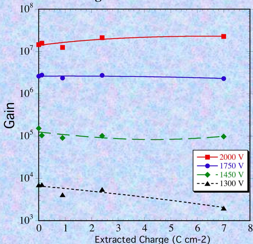
Gain stability of #164-163 MCP pair during conditioning, for various MCP voltage settings.
