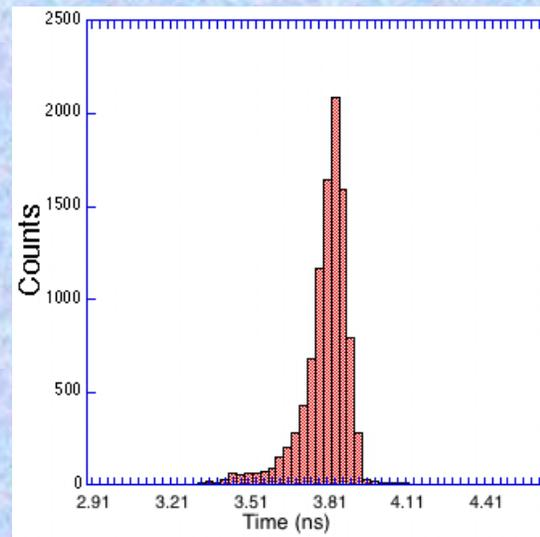
Laser ( $\sim 80 \text{ ps}$ ) measurements of timing jitter show 100ps time spread, 25mm cross delay line readout,  $10 \mu\text{m}$  MCP Z stack, S20 photocathode
