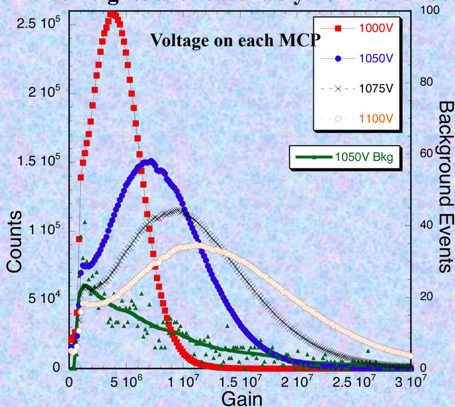
Pulse height amplitude distributions. MCP pair, 20 $\mu$ m pores, 8 $^\circ$  bias, 60:1 L/d, 0.7mm pair gap with 300V bias. 3000 sec background.
