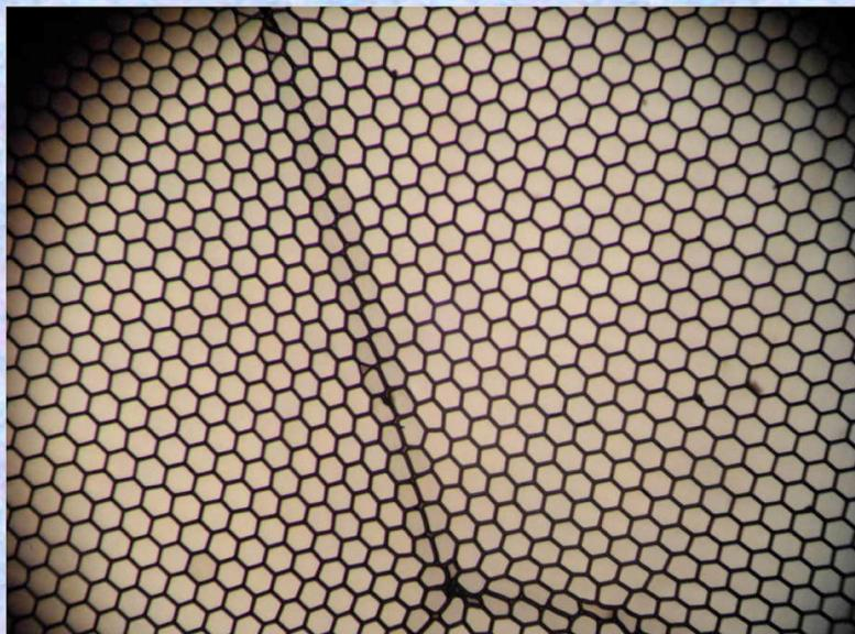
**Incom substrate, 40 $\mu\text{m}$  pores, 8 deg bias, 40:1 L/D, 83% OAR**
