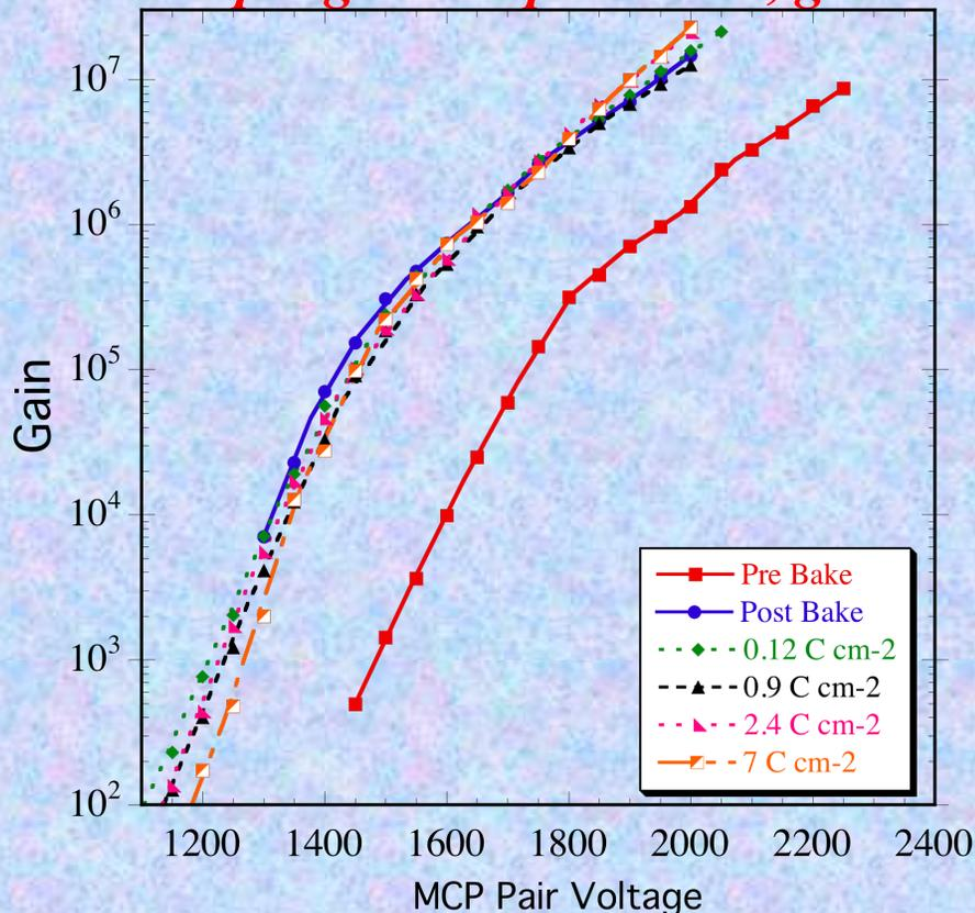
Gain curves of 164-163 MCP pair (20μm pore, 60:1 L/d, 8° bias) at stages during conditioning.
