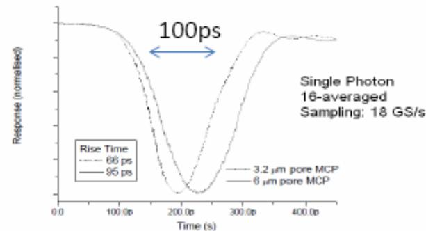
Time response curves for two models of PMT110 with different MCP pore diameters.
