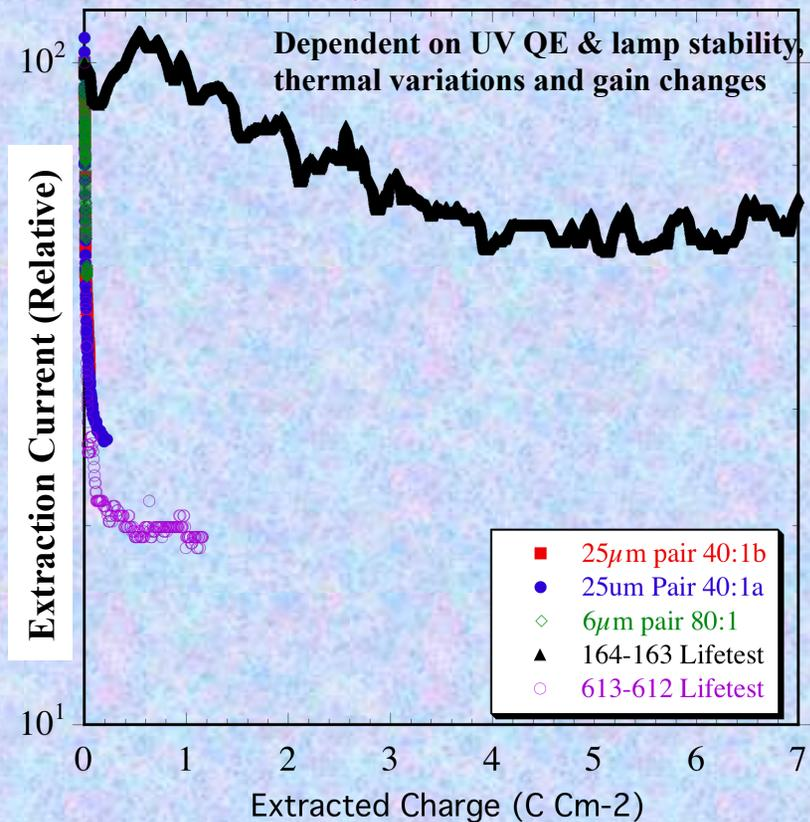
UV scrub of ALD MCP pair 164-163 (20μm pore, 60:1 L/d, 8° bias) compared with conventional MCPs. Outgas during burn-in < 4 x 10<sup>-10</sup> torr H<sub>2</sub>.
