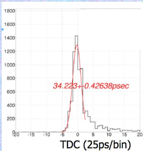
The transit time spread for single photoelectrons is  $\sim 30 \text{ ps}$ , this gets better with multiple photoelectrons ( $< 5 \text{ ps}$ )
