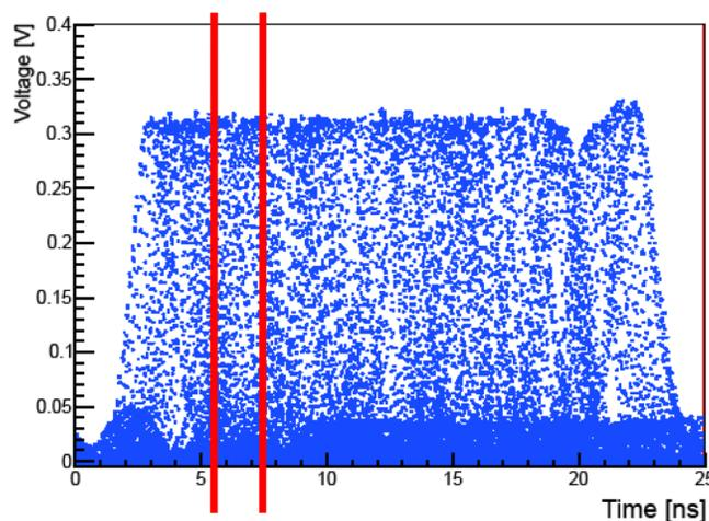
**2 channel timing (window subset - 3.8ps sigma)**
