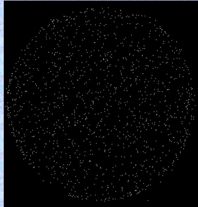
**3000 sec background, 0.0845 events cm<sup>-2</sup> sec<sup>-1</sup> at 7 x 10<sup>6</sup> gain, 1050v bias on each MCP. Get same behavior for most of the current 20 $\mu$ m MCPs.**
