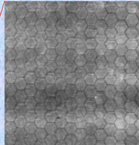
Image section showing the MCP multifibers
