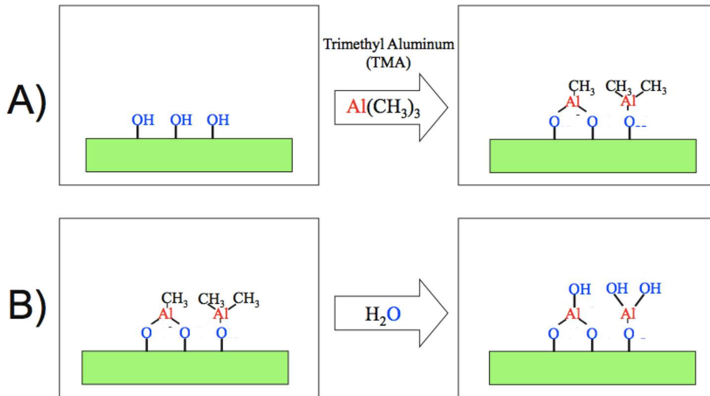
■ 1 ALD Cycle of TMA/ $\text{H}_2\text{O}$  Deposits 1  $\text{Al}_2\text{O}_3$  "Monolayer"
