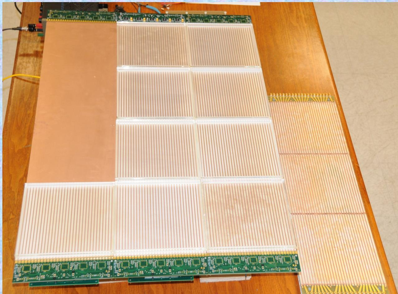
**Argonne 20cm glass tile package parts- anode, side-wall, windows
