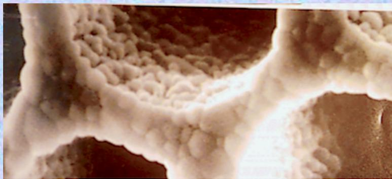
Opaque photocathode layer structure deposited onto microchannel plate
