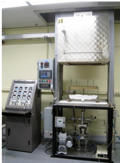
Figure 2. The PMT photocathode growth facility acquired from Photonis, installed at Argonne. Bi-alkali photocathodes with QE ~24% have been successfully grown at Argonne using this system.
