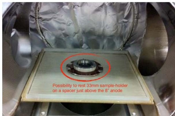
Fig. 1. Chamber for tests under vacuum with a  $20 \times 20 \text{ cm}^2$  glass tile patterned with transmission lines and a holder for a 33mm diameter MCP (mock tile MCP).
