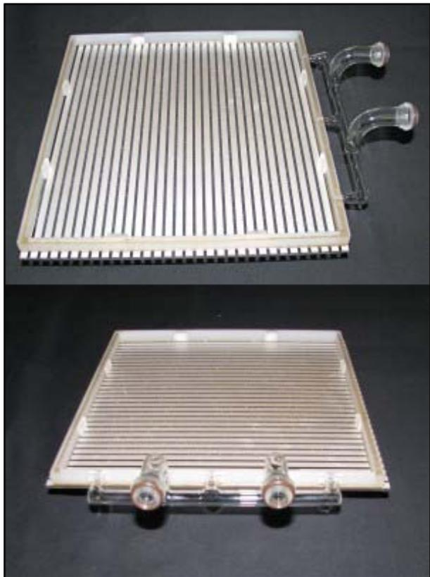
Fig. 2.  $20 \times 20\text{cm}^2$  vessel made of glass, and anodes.
