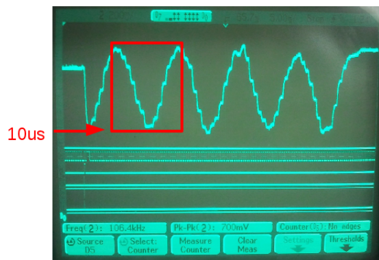
Figure 10: Analog voltage output with 100 MHz sine wave input. The input and output are analog voltages, so each step is quantized in time, hence the apparent steps.
