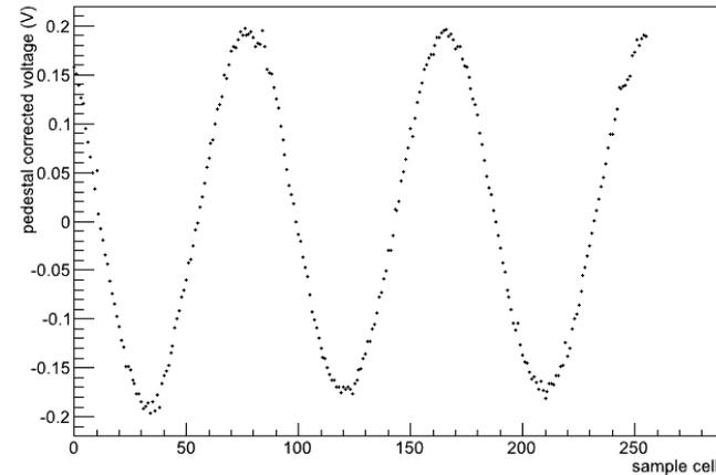
Visible attenuation along chip input
