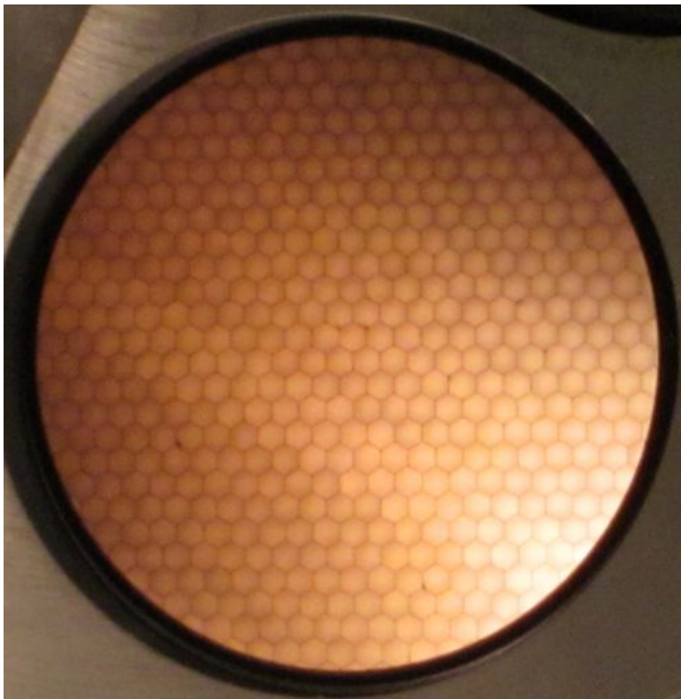
Visible light transmission for a 20 \mu\text{m} pore borosilicate micro-capillary ALD MCP .
