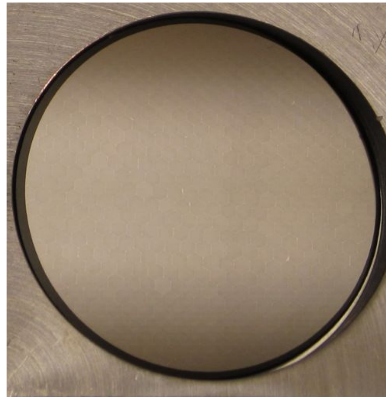
Surface photo for a 20 \mu\text{m} pore borosilicate micro-capillary ALD MCP with NiCr electrode .
