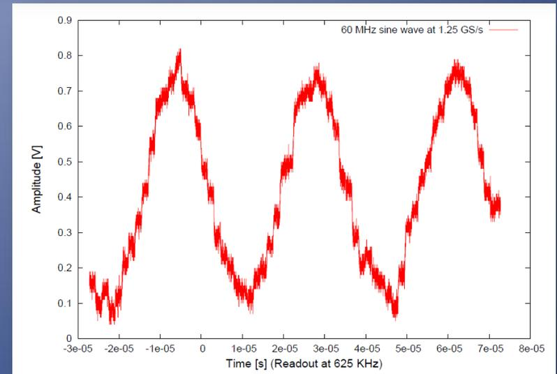
Analog outputs from Psec2 before correction showing cell-to-cell offset (and scope noise).
