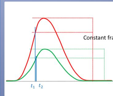
The constant fraction algorithm is very oftently used due to its relatively good results for and relative simplicity.
