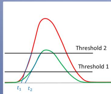
The multiple threshold method takes into account the finite slope of the signals. It is still very easy to implement.
