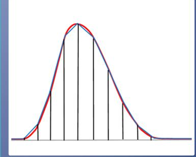
The waveform sampling above the Shannon frequency is the best algorithm since it is preserving the signal integrity.
