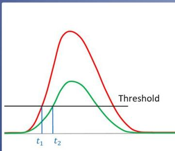
The single threshold is the least precise time extraction measurement. It has the advantage of simplicity.
