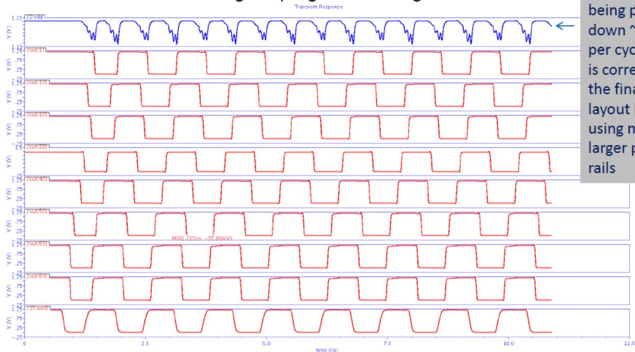
Note: vdd is being pulled down ~70 mV per cycle. This is corrected in the final ADC layout by using much larger power rails
